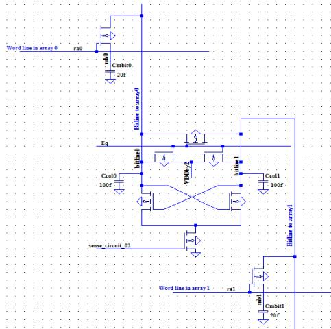
**Fig.7** Schematic for sense amplifier design topology 2
