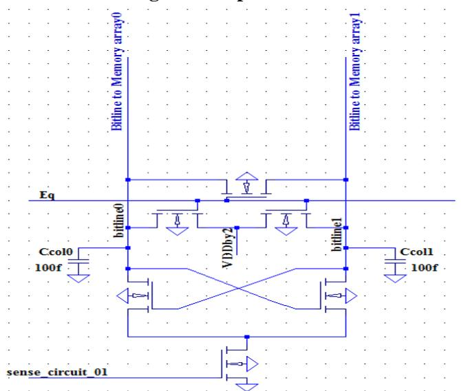
Fig.4 Schematic for sense amplifier design topology 1
