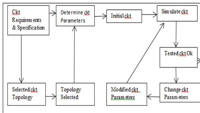
**Fig.3** Design procedure and methodology for various Topologies of sensing circuits
