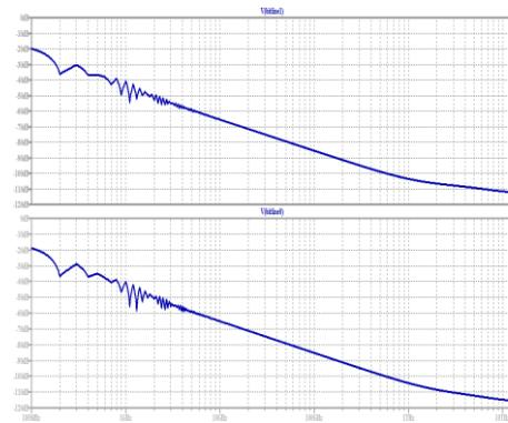
**Fig.6** FFT plot for topology1 bitline1 and bitline0 from 100 MHz to 10 THz
