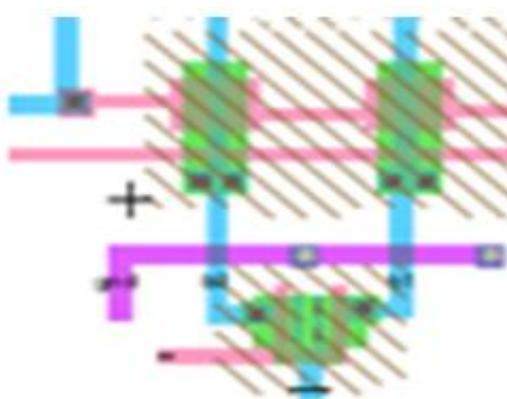
Fig.10 Layout view for sense amplifier interfacing to memory bit
