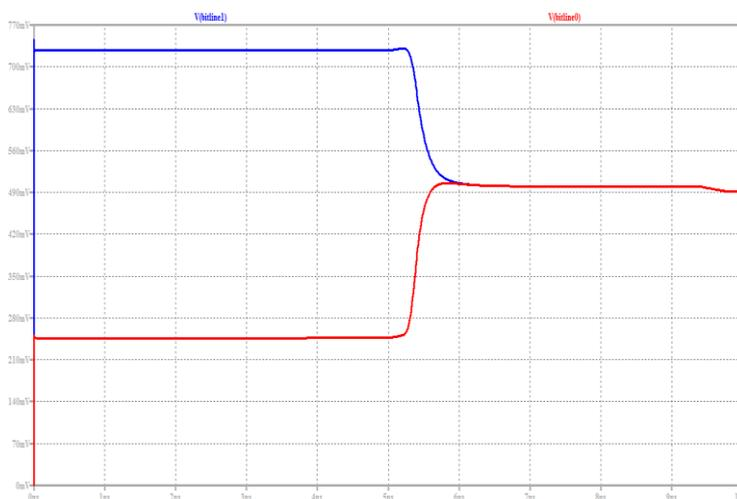
Fig.5 Transient simulation plot for bitline1 and bitline0
