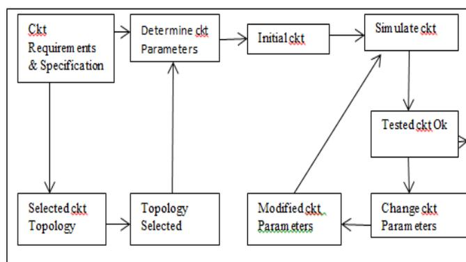
Fig.3 Design procedure and methodology for various Topologies of sensing circuits
