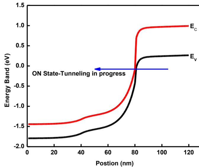
**Figure 3** Energy Band Diagram of designed DG heterostructure Tunnel FET
