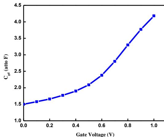
Figure 6 Gate-to-drain (C<sub>gd</sub>) capacitance at 4 nm dielectric thickness
