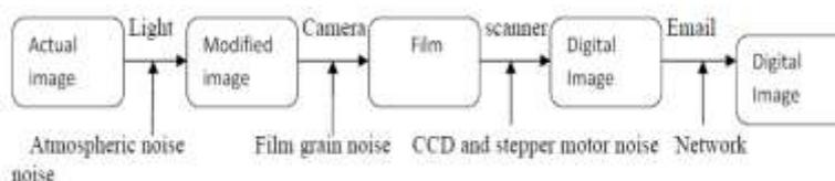
**Fig. 2.** Noise introduced at each step in the acquisition process.
