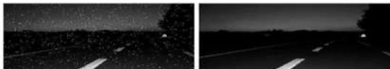
Fig 11: Image with impulse noise (Left) With Median Filter (Right)
