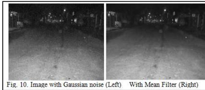
Fig. 10. Image with Gaussian noise (Left) With Mean Filter (Right)
