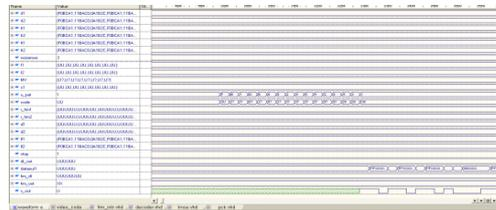
Figure 12: simulation result illustrating the generated code sequence for the coefficient compression
