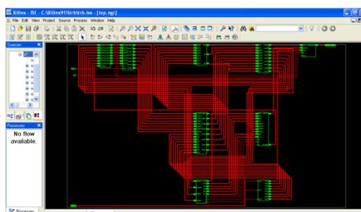
Figure 23: RTL view of the implemented system using Xilinx synthesizer.
