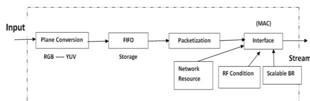
Figure 1: System Design for coding process in proposed architecture
