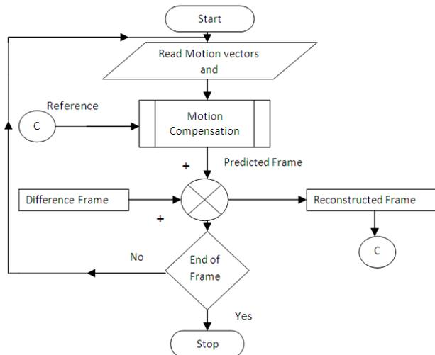
Figure 3 (b): Flowchart for Receiver block
