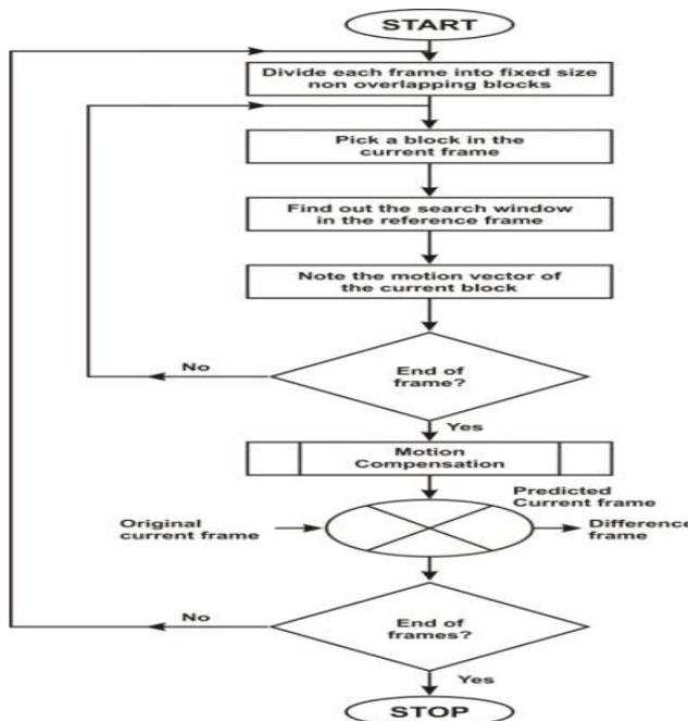
Figure 3(a): Flowchart for transmitter block
