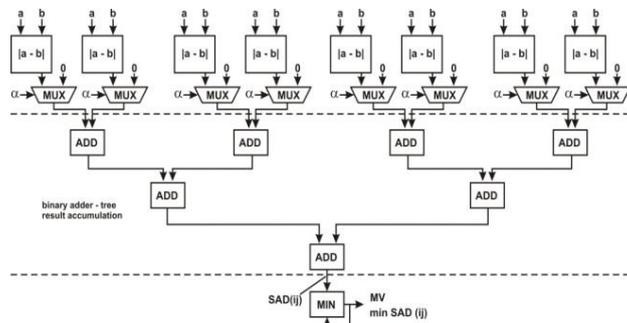
Figure 4: Digital model of matching algorithm for SAD calculation
