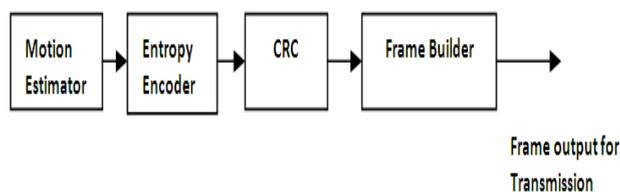
Figure 5: Video codec interface with motion estimator unit
