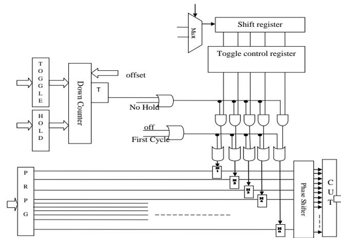
Figure 3 block diagram of Low Power Decompressor
