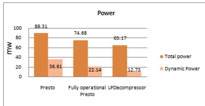
Figure 4 Power analysis of three various designs
