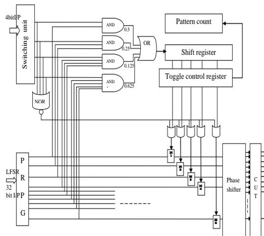
Figure 1 Block diagram of PRPG Operation
