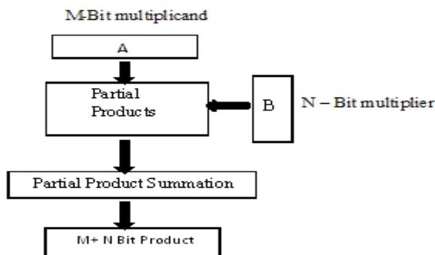
**Figure 1:** Multiplier Block Diagram
