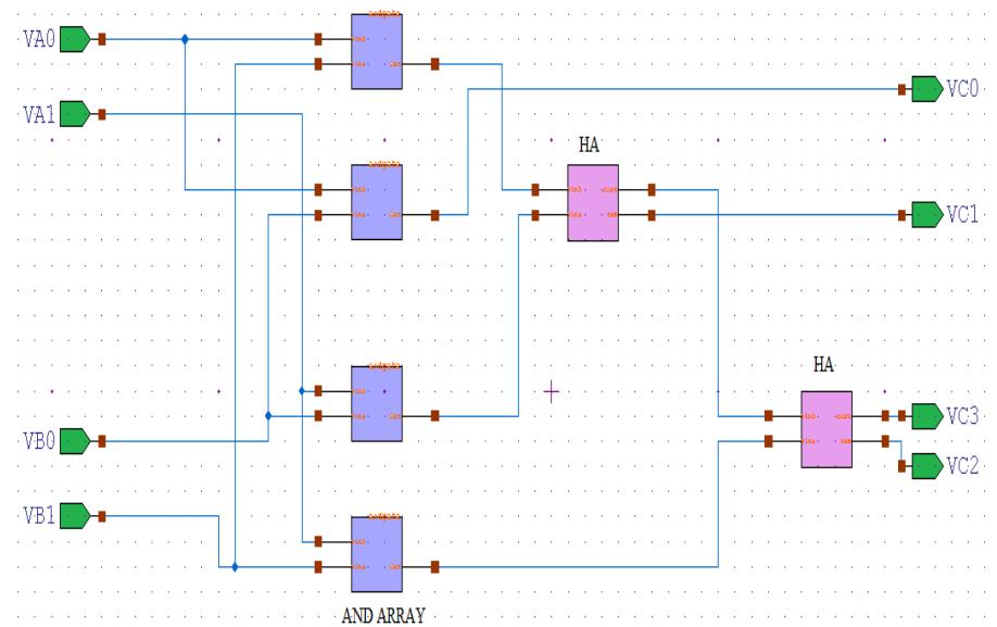
**Figure 4:** Schematic diagram of 2-bit multiplier
