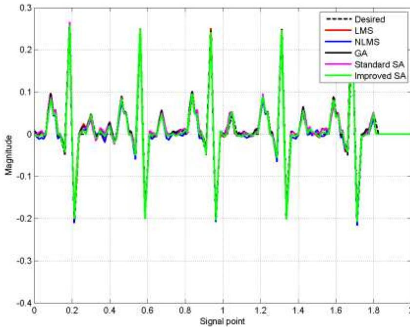
Fig. 12: LMS, NLMS, SA and improved SA algorithm results comparison
