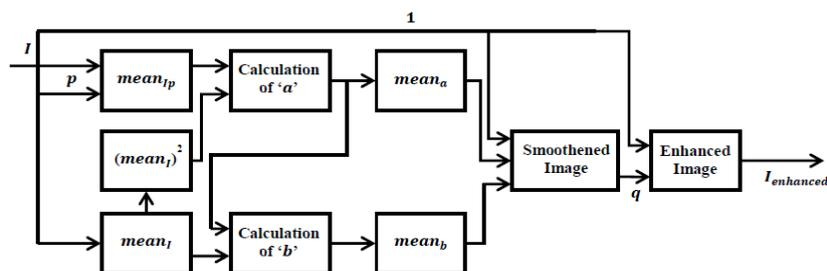
Fig.1.Internal block diagram of guided filter
