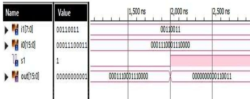
Fig .8.Simulation results for 2x1 multiplexer.
