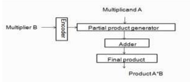
Fig.2. General block diagram of Booth multiplier.
