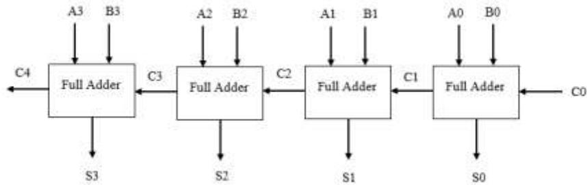
Fig.6. Ripple carry adder.
