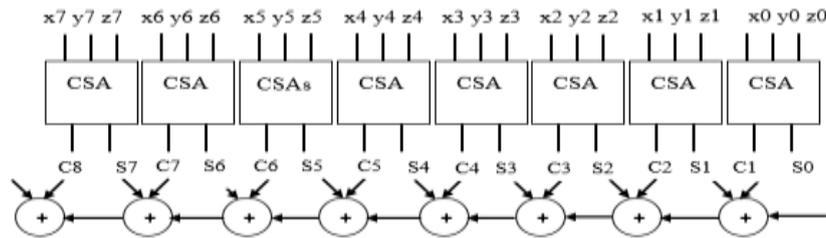
Fig.7. Architecture of Carry Save Adder.
