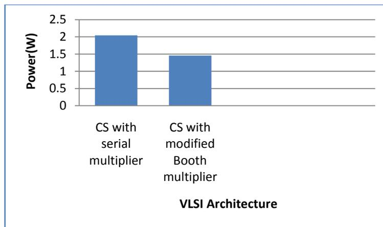
**Fig.15.** Power comparison of CS with serial multiplier and CS with modified Booth multiplier.
