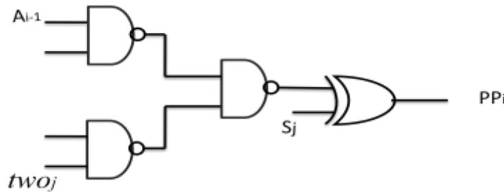
Fig.5. Block diagram of partial product generator.
