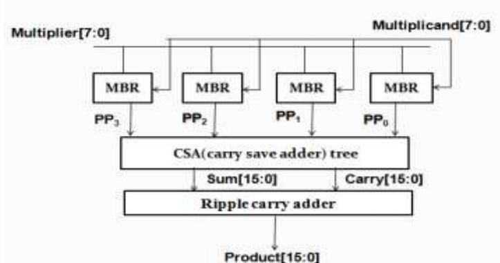
Fig.3. Block diagram of Radix-8 Booth algorithm.
