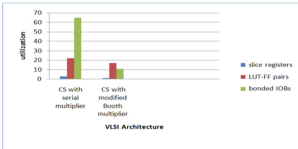
**Fig.16.** Comparison of area of CS with serial multiplier and CS with modified Booth multiplier.
