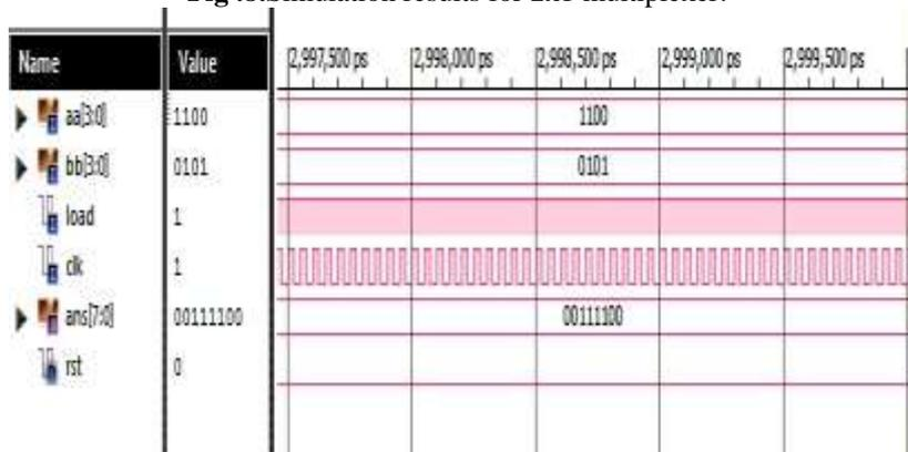
Fig .9. Simulation results for four bit serial multiplier.
