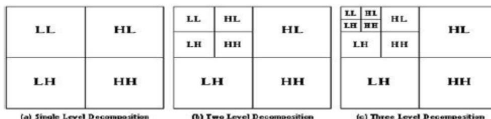
Fig2: Mechanism of daubechies wavelet.
