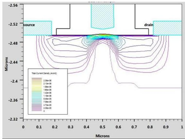
**Fig.9** Total Current Density of Si Control Pmosfet
