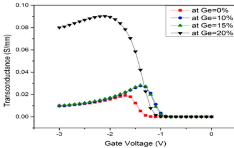
**Fig.8** Transconductance at different Ge Concentration
