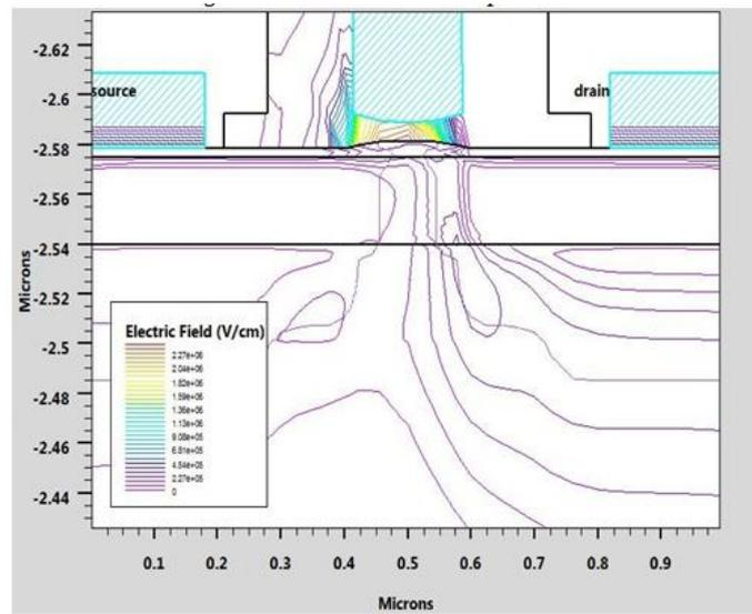
Fig.12 Electric field lines of Strained Si-pMOSFET
