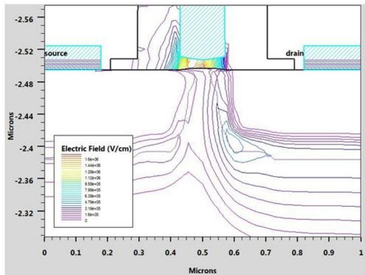
Fig.11 Electric field lines of Si-pMOSFET
