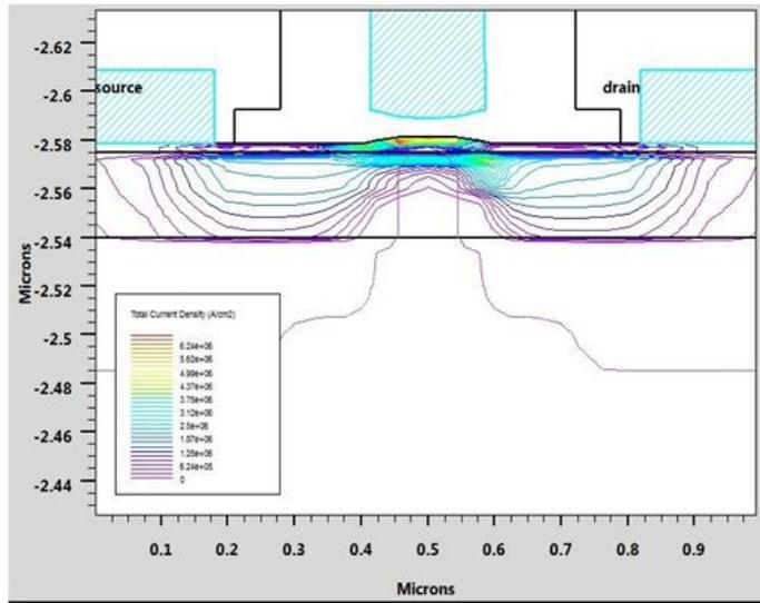
Fig.10 Total Current Density of Strained-Si pMOSFET
