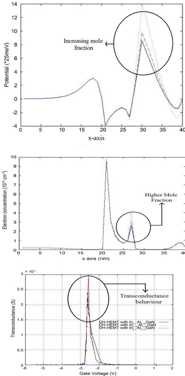
Fig 2 (a) Potential calibrated to 25mV showing increasing mole fraction, (b) Electron concentration of the device showing mole fraction, (c) Transconductance behavior with applied Gate voltage.
