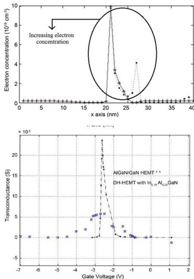
Fig 3 (a): Increasing concentration of electrons with respect to x-axis, (b) Transconductance of AlGaN/GaN HEMT against Gate voltage.
