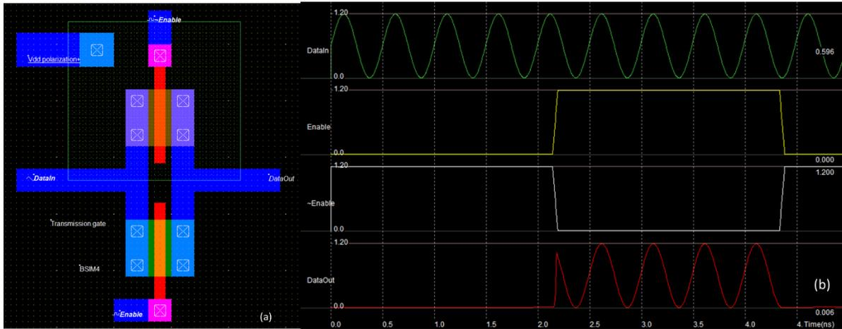
Fig. 21. (a) Layout of the transmission-gate. (b) Example simulation test for the function of transmission gate.
