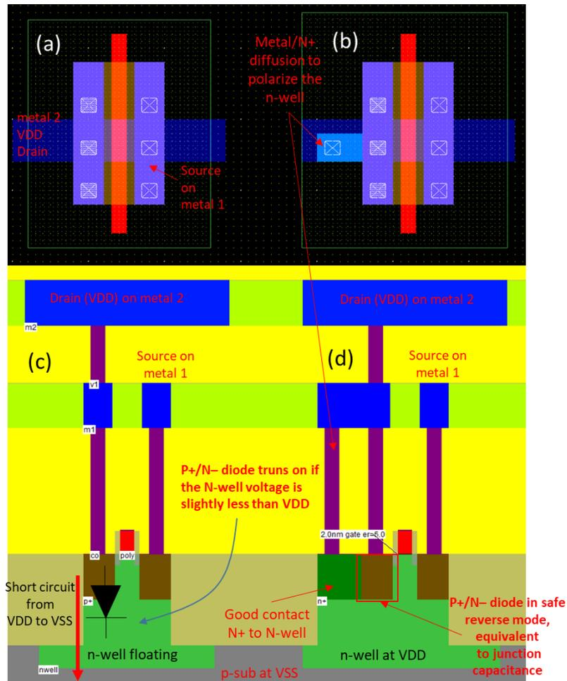
**Fig. 15.** (a) pMOS layout without n-well polarization. (b) pMOS layout with n-well polarization. (c) Cross-section of pMOS without n-well polarization. (d) Cross-section of pMOS with n-well polarization.
