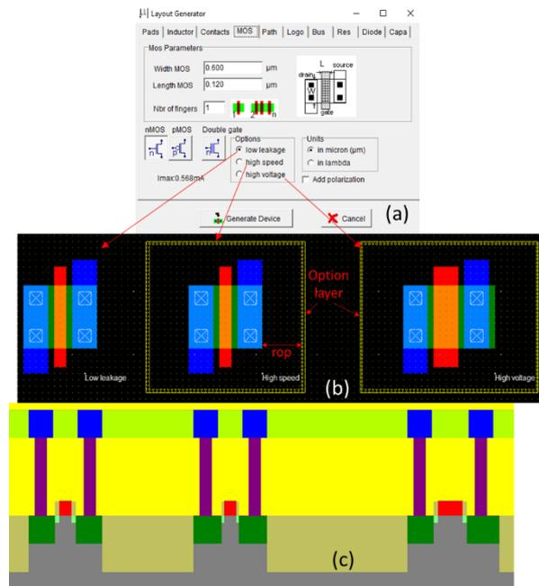
Fig. 11. (a) Layout generator, (b) top-down and (c) cross-section view of low leakage, high speed and high voltage nMOS device. In (b) also is shown the detailed top-down view of option-layer placement design rules.
