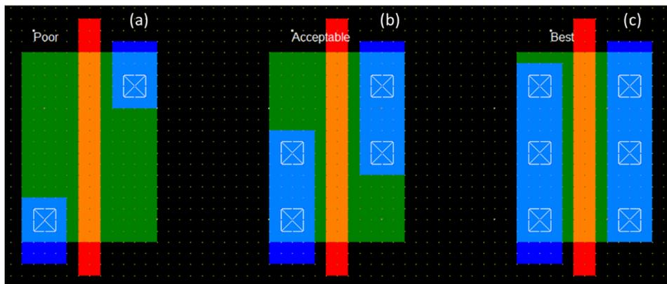
Fig. 14. Adding more contacts is desirable. (a) Poor nMOS design. (b) Acceptable nMOS design. (c) Best nMOS design.
