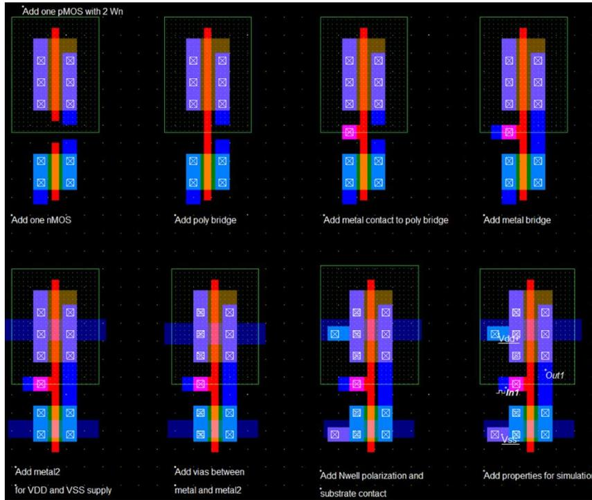
Fig. 19. Layout design steps for a CMOS not gate using 0.12µm technology.
