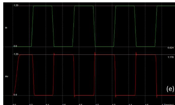
Fig 23. Timing simulation of CMOS inverter layout starting from its Verilog description.
