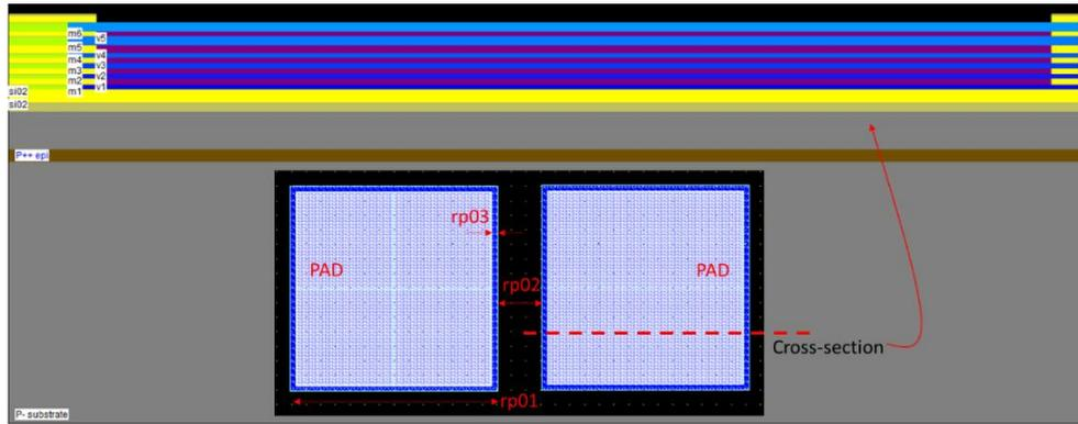
Fig. 10. Detailed top-down and cross-section view of basic PADS design-rules.
