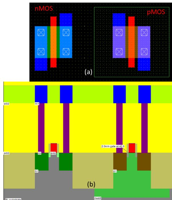
Fig. 12. nMOS and pMOS layout and cross-section view.
