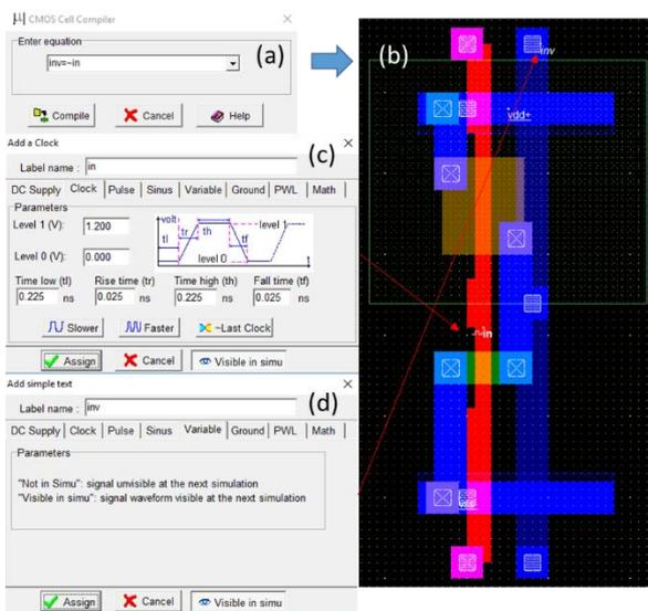
Fig. 22. (a, b) Creation of a CMOS inverter from its Verilog description. (c, d) Assigning simulation properties.
