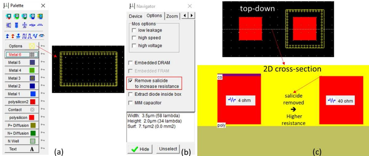
Fig. 4. (a). Option layer. It is a virtual layer (not a mask layer). (b, c). One of its properties is to remove the salicide to increase layer resistance.
