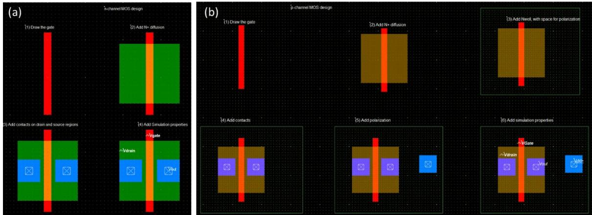
Fig. 13. Steps for custom design of MOS devices. (a) Simple nMOS. (b) Simple pMOS.
