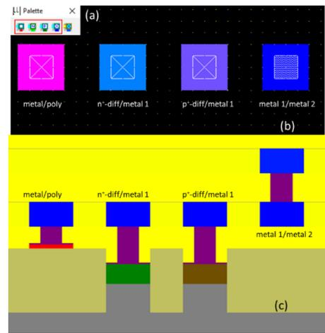
Fig. 2. Contacts in Microwind. Cross-section among various contacts.
