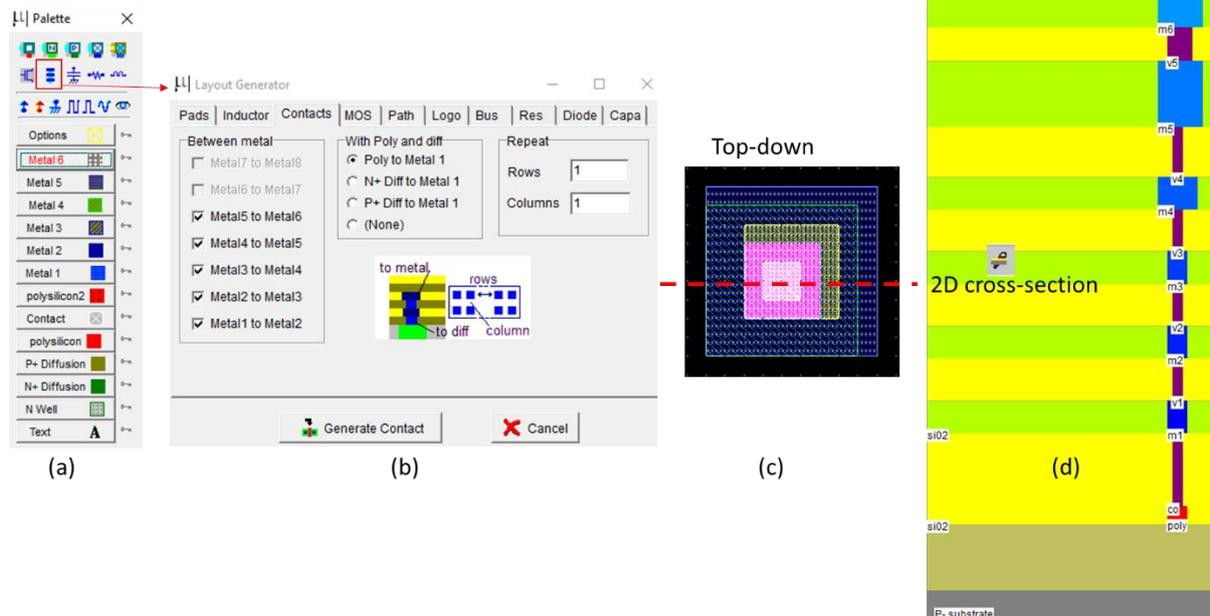
Fig. 3. Layout generator can be used to create complex contacts between various metal layers. Contacts of metals higher than metal 2 are larger.
