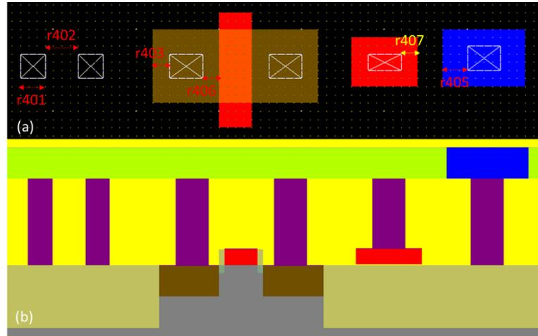
Fig. 8. Detailed top-down and cross-section view of contact (via) placement design rules.
