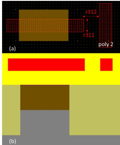
Fig. 7. Detailed top-down and cross-section view of polysilicon 2 placement design rules.
