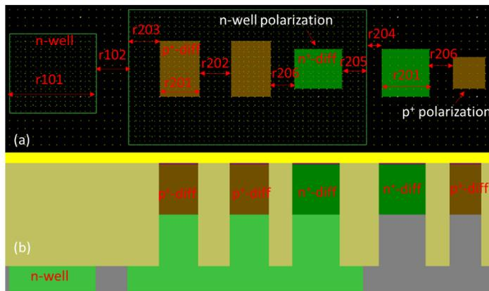
**Fig. 5.** Detailed top-down and cross-section view of n-well, n+, p+ diffusion placement design rules.
