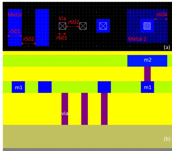
Fig 9. Detailed top-down and cross-section view of metal and via design-rules. Similar rules apply to higher metal layers and corresponding viases.
