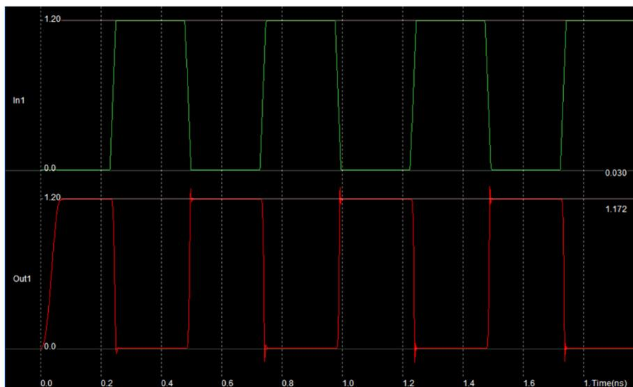
Fig. 20. Timing simulation of the CMOS not gate.
