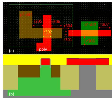
**Fig. 6.** Detailed top-down and cross-section view of polysilicon placement design rules.
