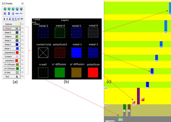
Fig.1. (a) Microwind's palette showing various layers and tools assisting layout design. (b)  $3\lambda \times 3\lambda$  squares are depicted one for each layer. Starting from n-well which is the deepest level, the layers become shallower as the series progresses to metal 6. (c) Cross-section among the various layers.
