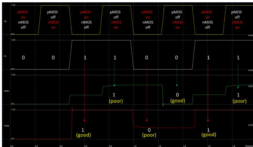
Fig. 18. Simulation of nMOS and pMOS dynamic behavior.
