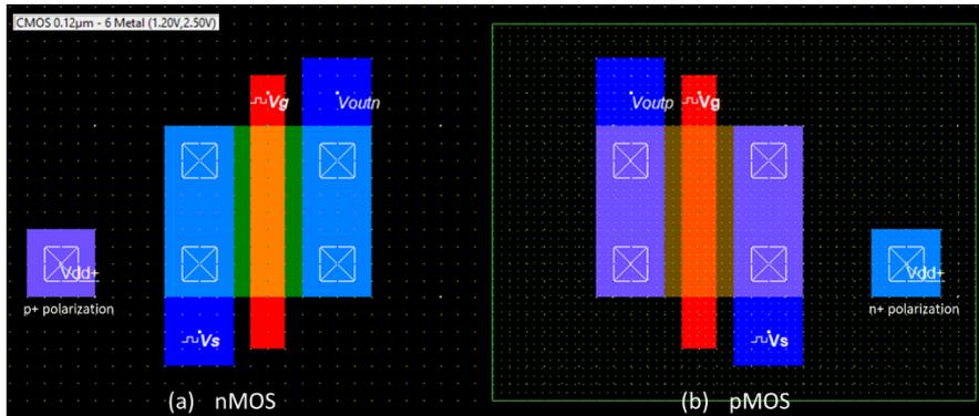
Fig. 16. (a) nMOS and (b) pMOS devices with added simulation properties and appropriate polarization.
