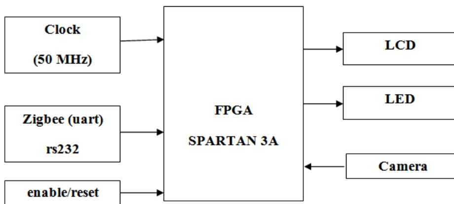
Figure 1. Proposed Parking Detection system on Spartan FPGA
