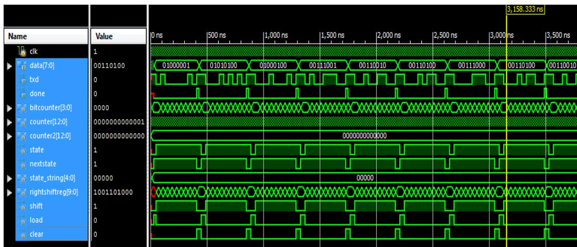
Figure 8. Transmitter module for UART communication
