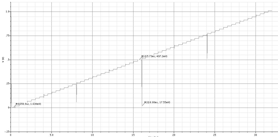
**Figure 16.** 6-bit 1-MSB PBTN output waveform of this work.
