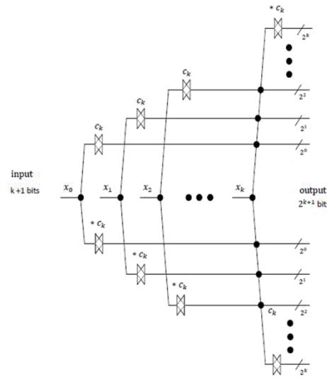
**Figure 4.**  $k+1$  bit 1-MSB PBTN [3]
