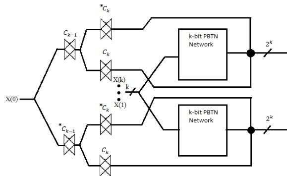
**Figure 5.**  $k+1$  bit 2-MSB PBTN [3]
