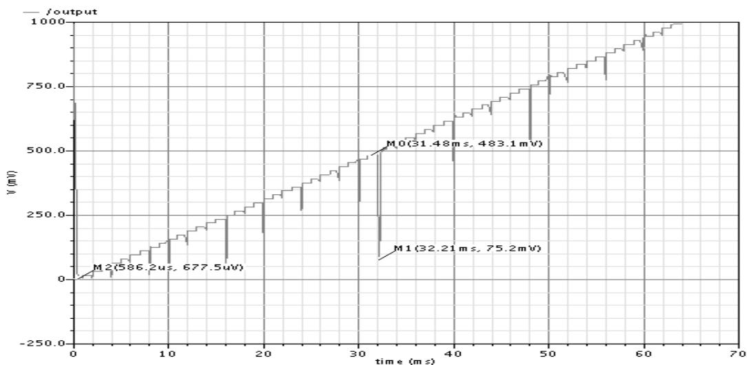
**Figure 15.** 6-bit 1-MSB PBTN output waveform from work in [2].
