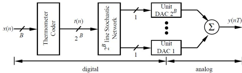
**Figure 2.**General topology of a B-bit stochastic DEM DAC [5].
