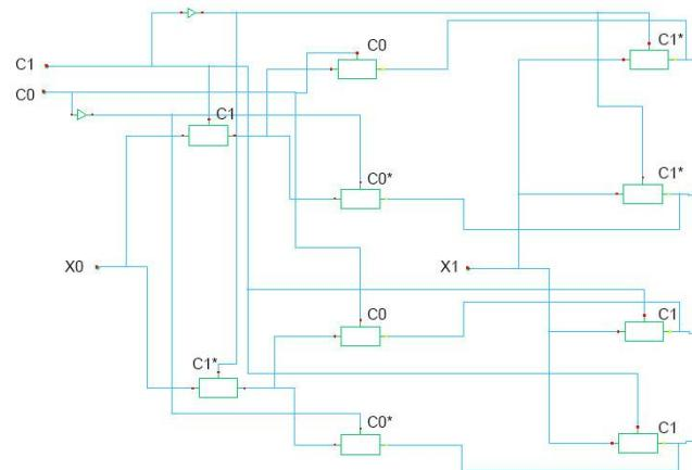
**Figure 9.** 2-bit 2-MSB PBTN design
