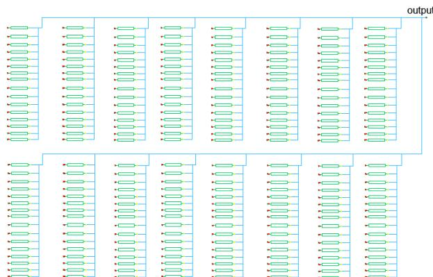
**Figure 13.** 8-bit current steering DAC using 256 current sources
