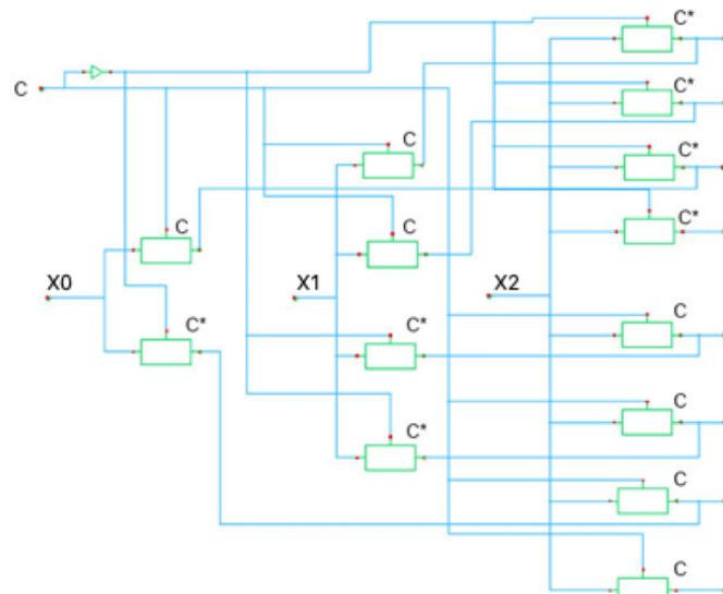
**Figure 7.**3-bit 1-MSB PBTN design
