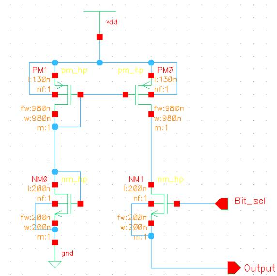
**Figure 12.** Simple switchable current source
