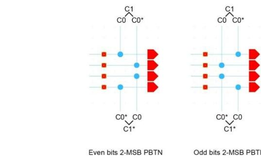
**Figure 11.2-MSB k+1 bit transmission gate to output connections**
