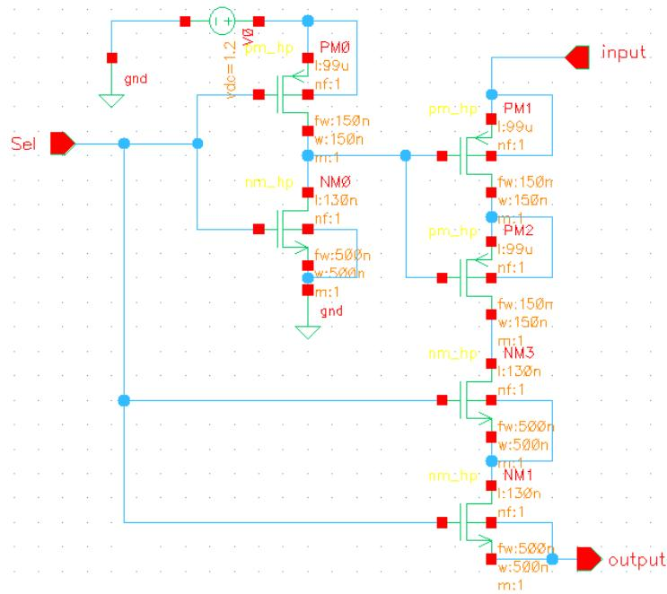
**Figure 6.**An optimized schematic design of transmission gate
