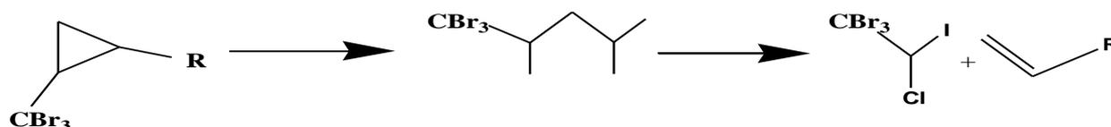
Scheme 2. Retrosynthetic Pathway for the Synthesis of Tribromomethyl-Substituted Cyclopropanes from CBr<sub>3</sub>CHICl
