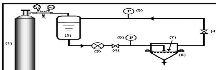
**Fig 1:** Diagram of the pilot of filtration: (1) nitrogenBottle (2)Water tank (3)circulating pump(4) valves(5) manometers (6)Modulates membrane (7) membrane.
