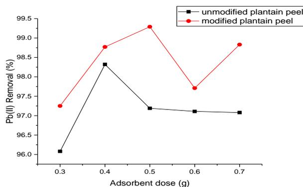
**Figure 4:** Effect of increase in adsorbent dosage on the percentage removal of lead ions.
