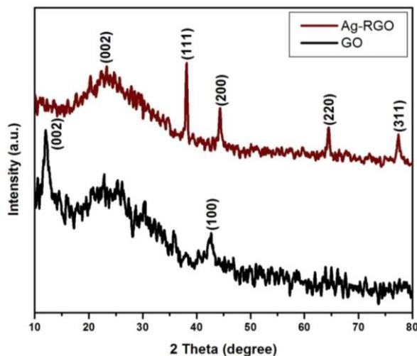
Fig.1. XRD patterns of GO and Ag-RGO nanocomposite.
