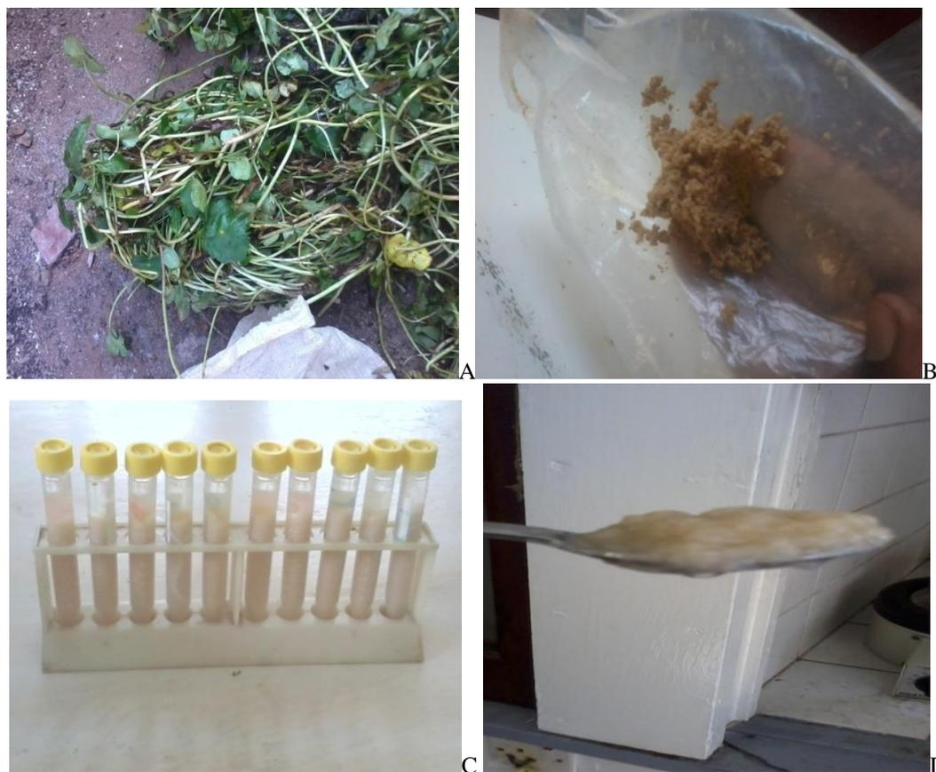
**Figure 1.** Photographs of some of the steps (A) raw sample (B) alkali treated (C) after centrifugation (D) after acid hydrolysis.
