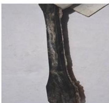
**Figure 6:** 20% Starch + 80% PE after 60days
