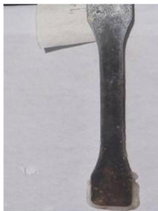
**Figure 5:** 15% Starch + 85% PE after 60 days.
