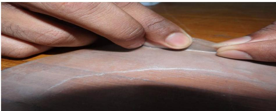
**Figure 20:** 0% Starch-PE Film Resistant to Tear
