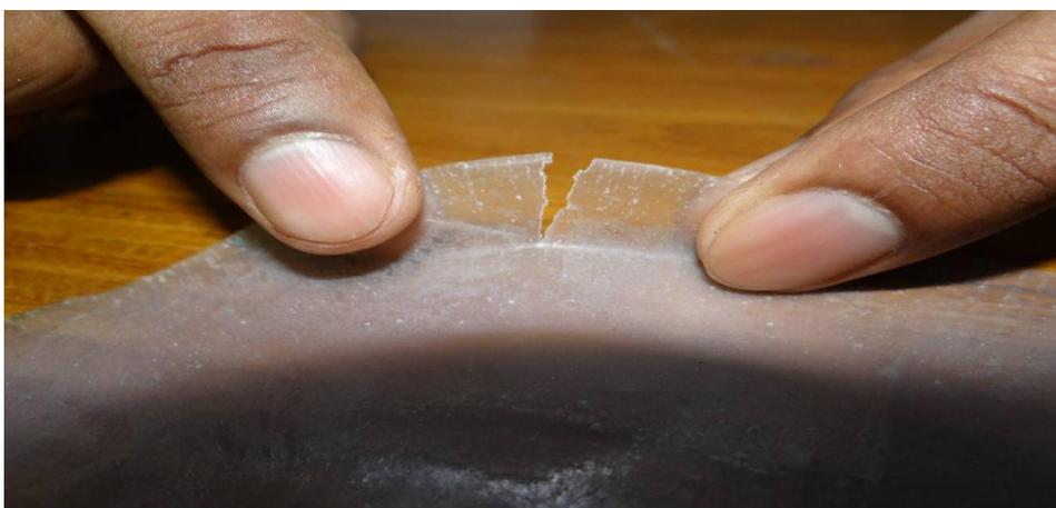
**Figure 21:** 10% Starch-PE Film Easier to Tear
