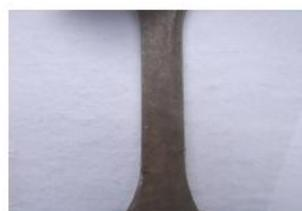
**Figure 3:** 5% Starch + 95% PE after 60 days
