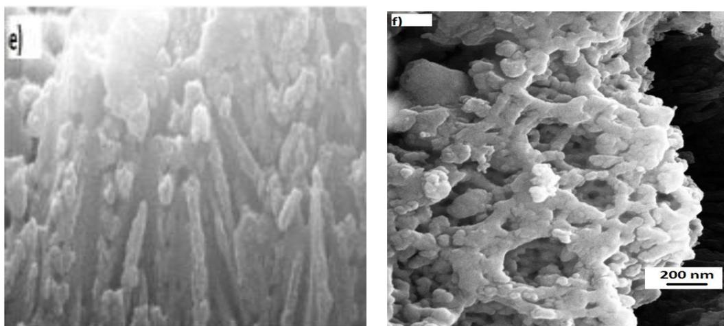
**Figure 3.** FE-SEM cross-sectional view micrographs of nanowires anodized at 150 V in 0.3 M  $H_3PO_4$  for 1 hr at 30 °C e) Iron Nanowires at dc electrodeposition f) nanoclusters after 5 minutes at a scale of 200 nm.
