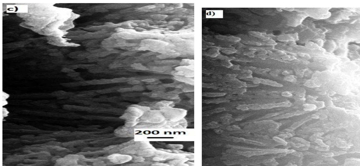
**Figure 2.** FE-SEM cross-sectional view micrographs of nanowires anodized at 150 V in 0.3 M  $H_3PO_4$  for 1 hr at  $30^\circ C$  Iron Nanowires at ac electrodeposition at a scale of 200 nm
