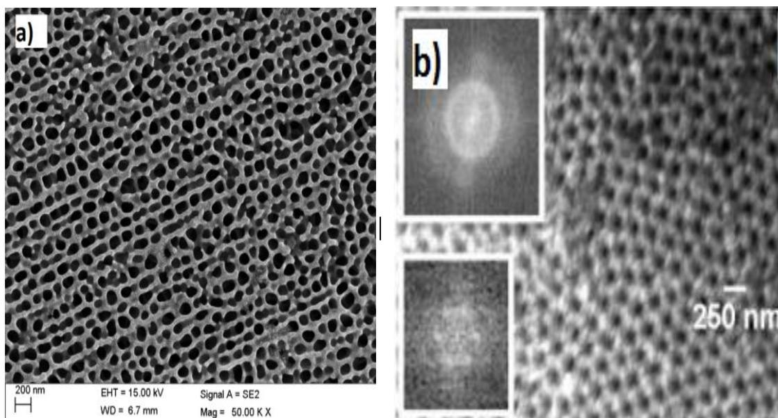
**Figure 1.** FE-SEM top view micrographs for anodized samples at 150 V in 0.3 M  $H_3PO_4$  for 1 hr at  $30 \pm 5^\circ C$  at a scale of a) 200nm b) 250 nm with FFT showing regularity of pores.
