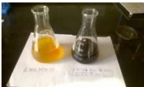
Figure1. Picture of C. papaya leaf extract with 1 mm \text{AgNO}_3 solution before and after the CPL-AgNPs.
