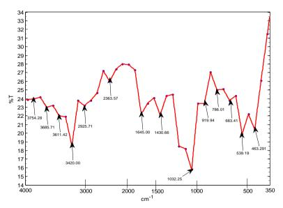
Figure 4 FTIR spectrum of Sphagnum cymbifolium(moss) before adsorption
