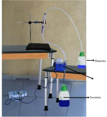
Figure 1 Fixed bed technique apparatus
