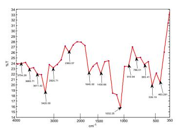
Figure 7: FTIR spectrum of Sphagnum cymbifolium (moss) before adsorption
