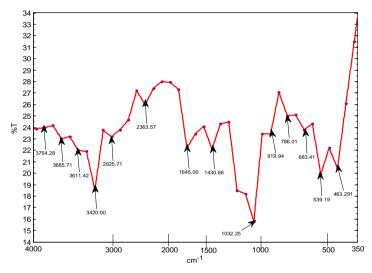
Figure 9: FTIR spectrum of Sphagnum cymbifolium(moss) before adsorption
