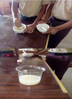
b. Take a beaker and add 200ml Diluted juice of Carambola. We used two electrodes of copper and zinc in here. We emerge two electrodes in the solution such a way that they could not touch each other. An electric wire is connected between them.
