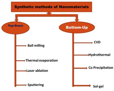
Figure 1: Synthesis of nanomaterial Approaches.
