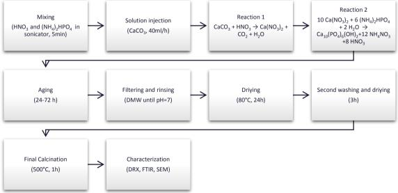
Figure 5. Sol-Gel process for HAP production using organic waste.
