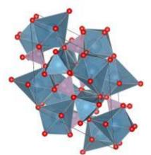
Figure 1. Crystalline structure for hydroxyapatite
