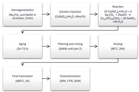
Figure 4. Sol-Gel process for HAP production using synthetic precursors.
