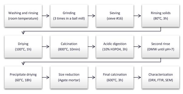
Figure 6. Sol-GEL process for PAH production using marine animal exoskeletons.
