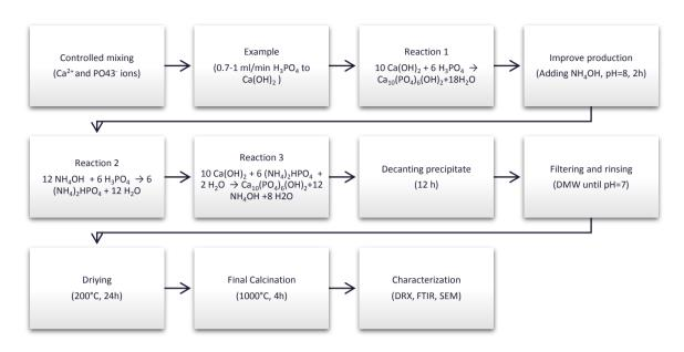
Figure 2. Chemical precipitation process for HAP production
