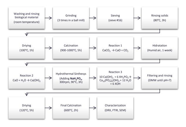
Figure 3. Hydrothermal process for HAP production
