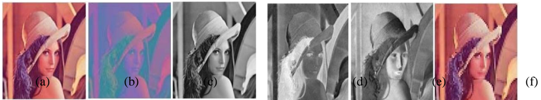
Figure 4: (a) Original image (b) YCbCr image (c) Y-component (d) Cb-component (e) Cr-component (f) Restored image with threshold 8 of CR=1.8895 and PSNR=32
