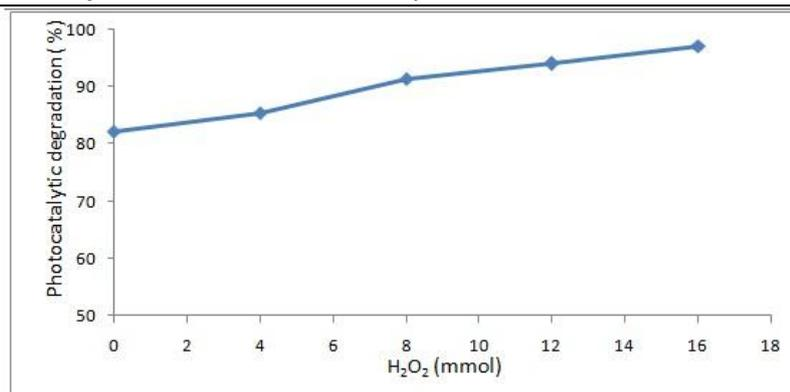
Fig. 7. Effect of addition of H<sub>2</sub>O<sub>2</sub> concentration on the degradation of 4-NP using solar light ZnPc/TiO<sub>2</sub> = 100 mg/100 ml; [4-NP] = 1 × 10<sup>-4</sup> M; pH 6.0±0.1; irradiation time = 60 min.
