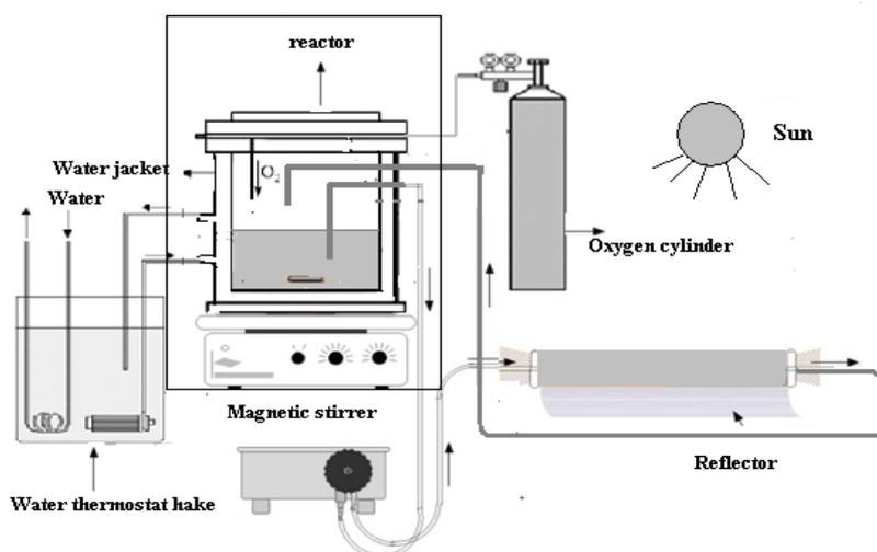
Fig. 2. Schematic diagram of the solar photocatalytic reactor system.
