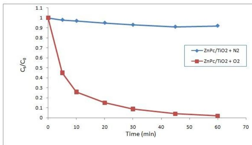
Fig. 6. Effect of type of gas on the degradation of 4-NP using solar light ZnPc/ TiO<sub>2</sub> = 100 mg/100 mL; [4-NP] =  $1 \times 10^{-4}$  M; pH 6.0±0.1; irradiation time = 60 min.
