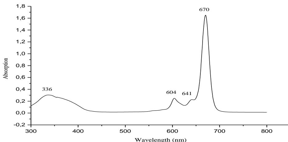
Fig. 1. UV-Vis spectrum of ZnPc in DMF solution at room temperature.
