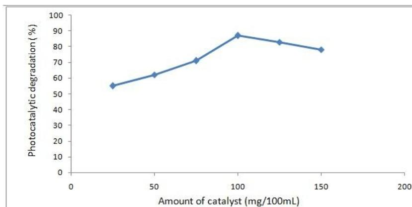
Fig. 5. Effect of catalyst weight on the degradation of 4-NP using solar light; [4-NP] =  $1 \times 10^{-4}$  M; pH  $6.0 \pm 0.1$ ; irradiation time = 60 min.
