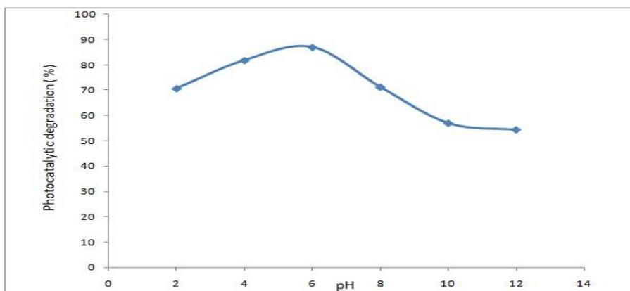
Fig. 4. Represent the effect of change in pH on photocatalytic degradation of 4-NP using solar light.
