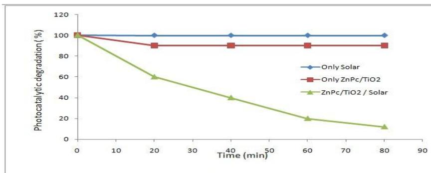
Fig. 3. Effect of solar light and ZnPc/TiO<sub>2</sub> on photocatalytic degradation of 4-NP [4-NP] = 1 × 10<sup>-4</sup> M; pH 6.0 ± 0.1.
