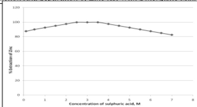
Fig. 2: Extraction behavior of Zinc (II) with synergistic mixture of N-n-octylaniline and Trioctylamine in xylene as a function of concentration of sulphuric acid at 0.25M potassium thiocyanate.
