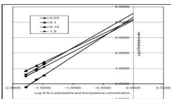
Fig. 5: Distribution Ratio of Zinc (II) as function of synergistic mixture of N-n-octylaniline and Trioctylamine concentration at 0.03, 0.1, 0.15 and 1.5 M potassium thiocyanate concentration.
