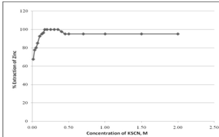
Fig. 1: Extraction behavior of Zinc (II) with 1% synergistic mixture of N-n-octylaniline and Trioctylamine in xylene as a function of thiocyanate at 2.5M sulphuric acid.
