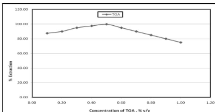
Fig. 3: Extraction behavior of Zinc (II) at fixed concentration of N-n-octylaniline (0.5%), by varying the concentration of Trioctylamine (TOA).
