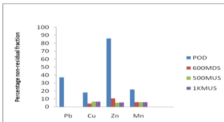
Figure 7: Comparing the residual fractions of Pb, Cu, Zn and Mn in samples collected at POD, 600MDS, 500MUS and 1KMUS
