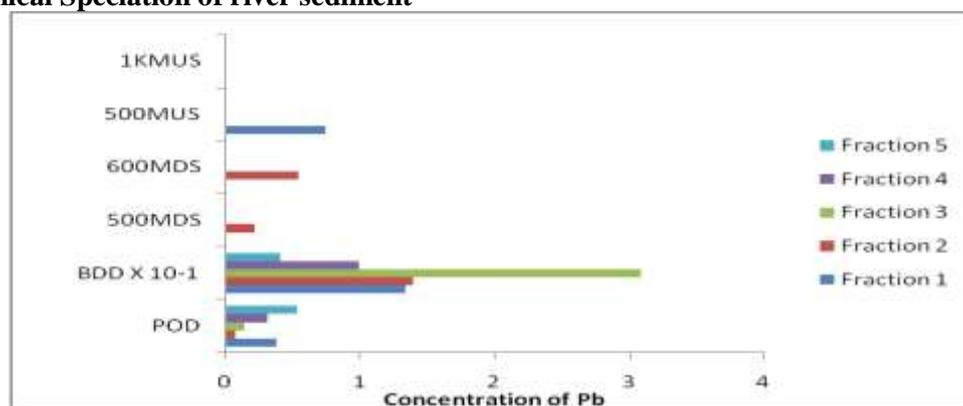
**Figure 1: Pb concentration (mg/kg) in various fractions of sediment samples**
