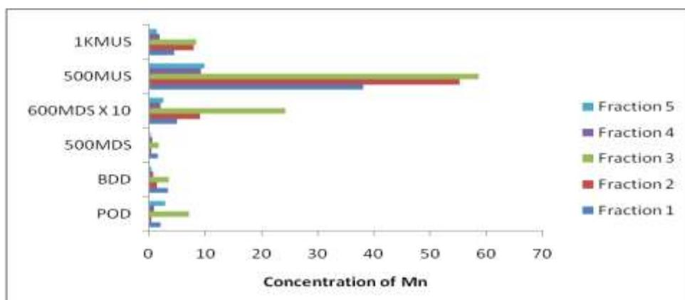
**Figure 4: Mn concentration (mg/Kg) in various fractions of sediment samples**
