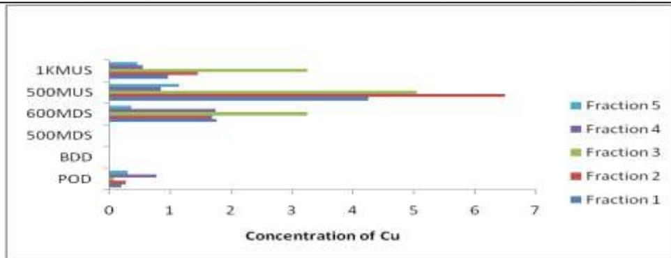
**Figure 2: Cu concentration (mg/Kg) in various fractions of sediment samples**
