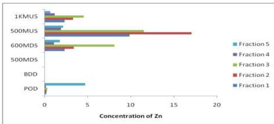
**Figure 3: Zn concentration (mg/Kg) in various fractions of sediment samples**
