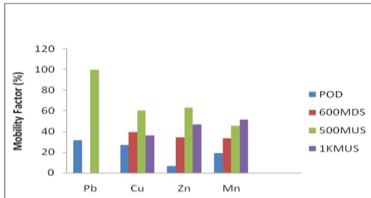
Figure 5: Comparing the percentage mobility of Pb, Cu, Zn and Mn in samples collected at POD, 600MDS, 500MUS and 1KMUS.
