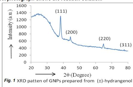
Fig. 1 XRD pattern of GNPs prepared from (±)-hydrangenol
