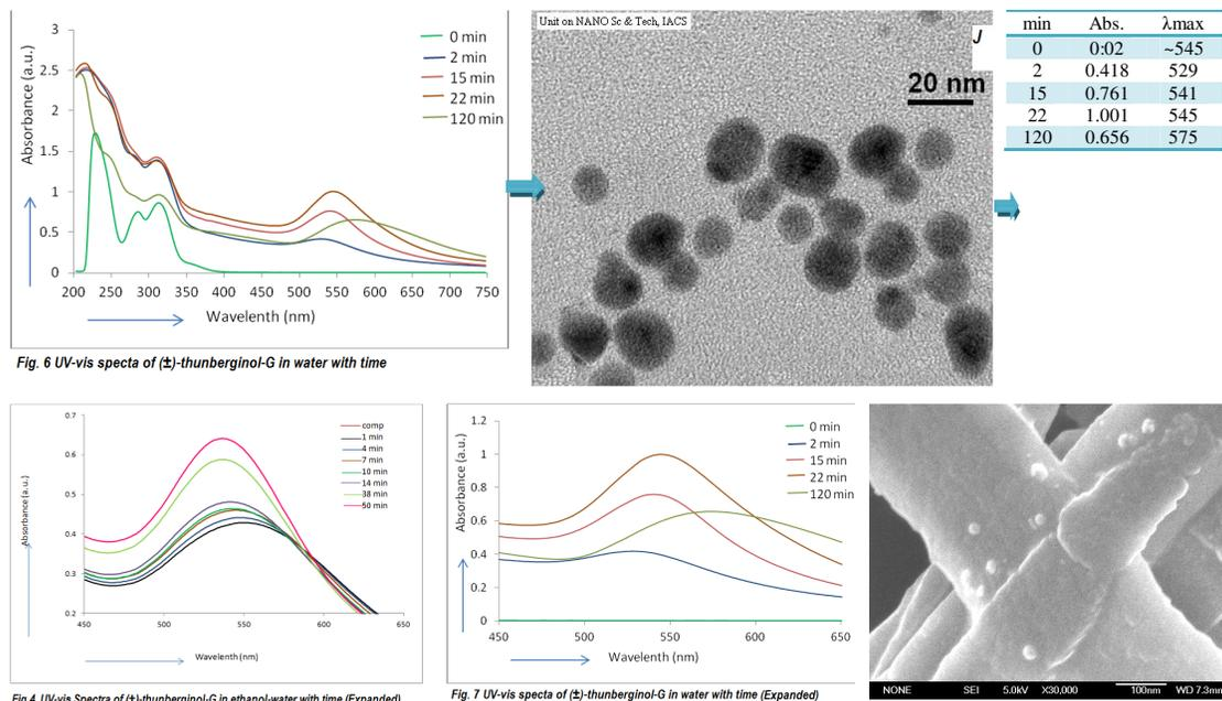
**Fig. 3, 4, 5, 6** represents UV-Vis spectra of GNPs synthesized/stabilized by (±)-thunberginol-G
