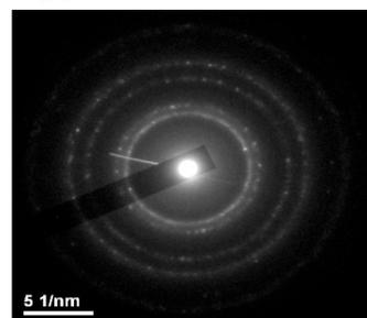
Fig. 2 SAED pattern recorded from GNPs shown in Fig. D
