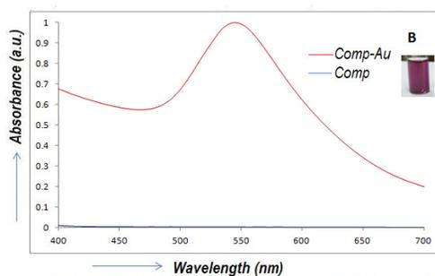
UV-visible absorption spectra of as-prepared gold nanoparticles. Inset photograph shows the reaction solution.
