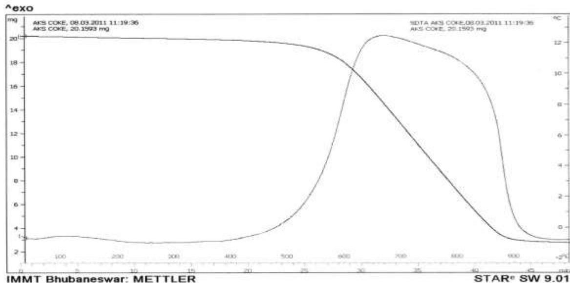
**Figure 3:** Differential thermal analysis of SPL carbon powder (Reference: graphite)
