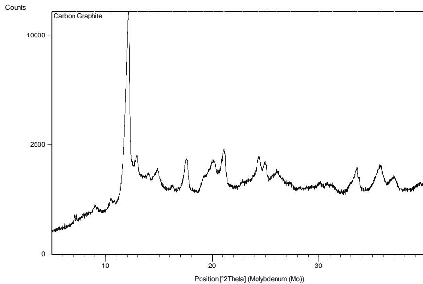
**Figure 1:** X-ray diffraction of SPL derived carbon powder
