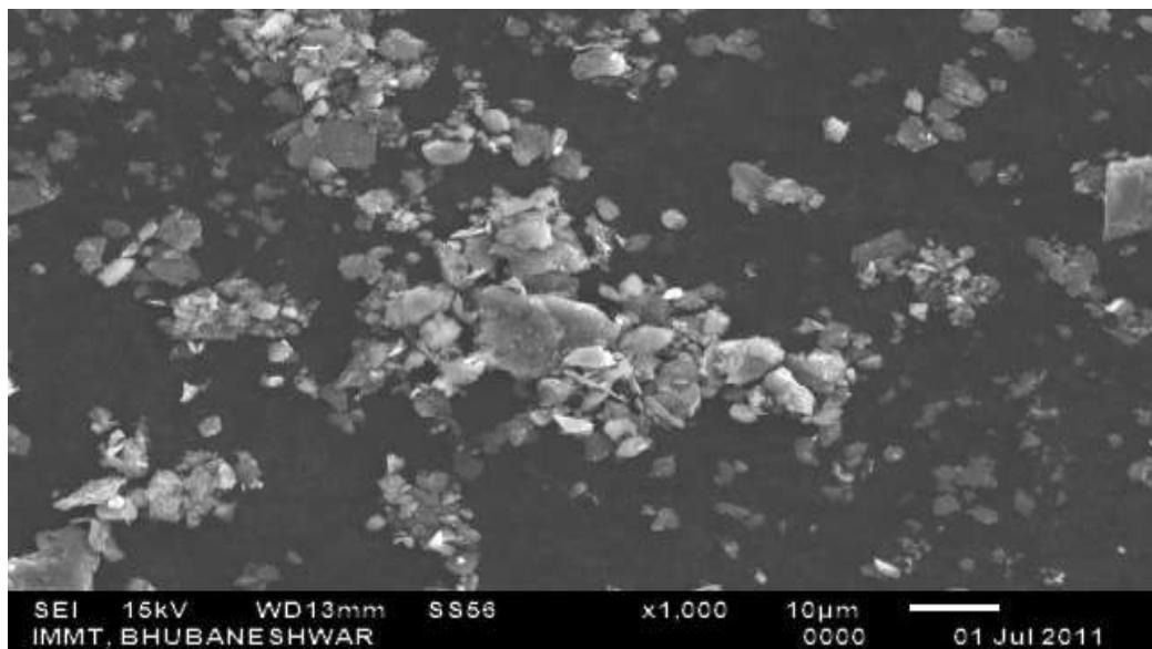
**Figure 2:** Scanning electron micrograph of SPL carbon powder.
