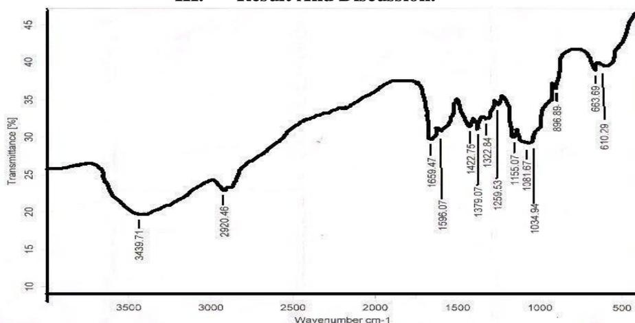
Fig 2: IR spectra of sorption of Cu(II) on chitosan
