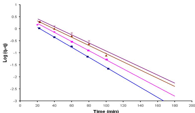
**Fig 4: Lagergren plot for the sorption of Cu (II) on chitosan:**
