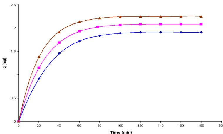
**Fig 5: Effect of temperature on the sorption of Cu (II) on Chitosan** ● 30°C, ■ 40°C, ▲ 50°C
