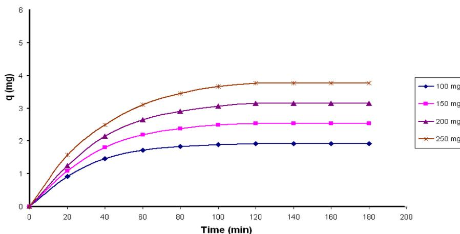
Fig 3 : effect of concentration for the sorption of copper (II) on chitosan;
