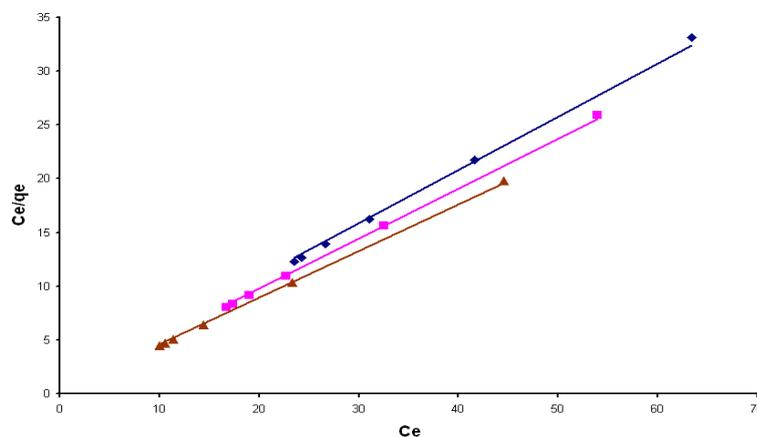
Fig 6: Langmuir isotherm for the sorption of Cu (II) on chitosan; ● 30°C, ■ 40°C, ▲ 50°C.
