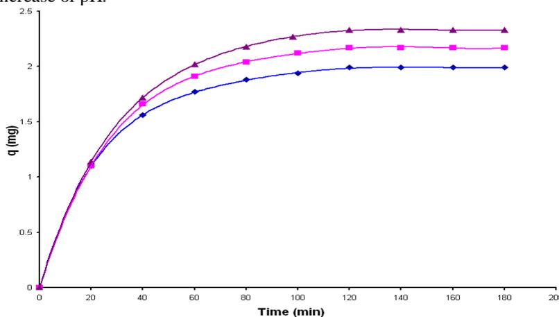
Fig 7: Effect of pH on the sorption of Cu(II) on chitosan; ● 2.0, ■ 4.0, ▲ 6.5; temp: 30 ° c, conc. 100 mg/l.
