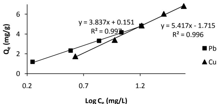
Figure 9: Temkin isotherms for the adsorption of Pb<sup>2+</sup> and Cu<sup>2+</sup> on shells of baobab
