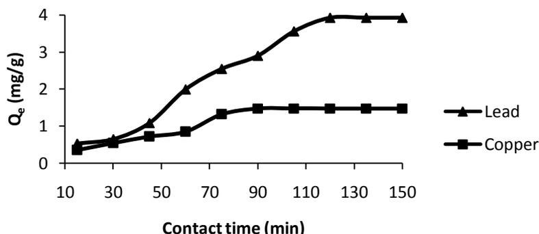
Figure 4: Effect of contact time on the sorption of  $\text{Cu}^{2+}$  and  $\text{Pb}^{2+}$  ions
