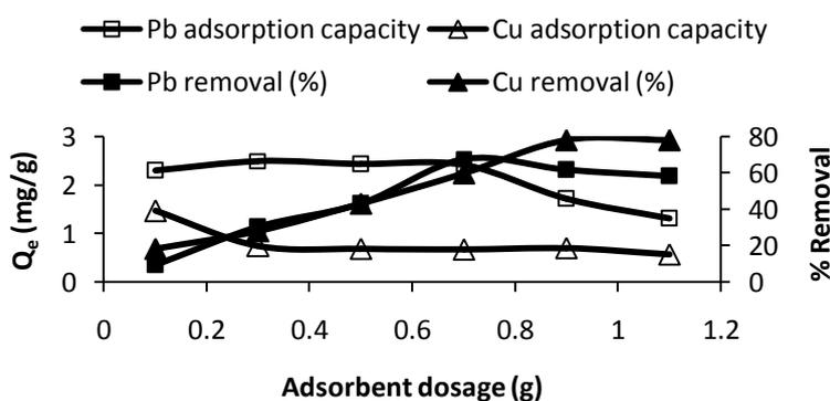
Figure 5: Effect of adsorbent dosage on adsorption of  $\text{Cu}^{2+}$  and  $\text{Pb}^{2+}$  ions
