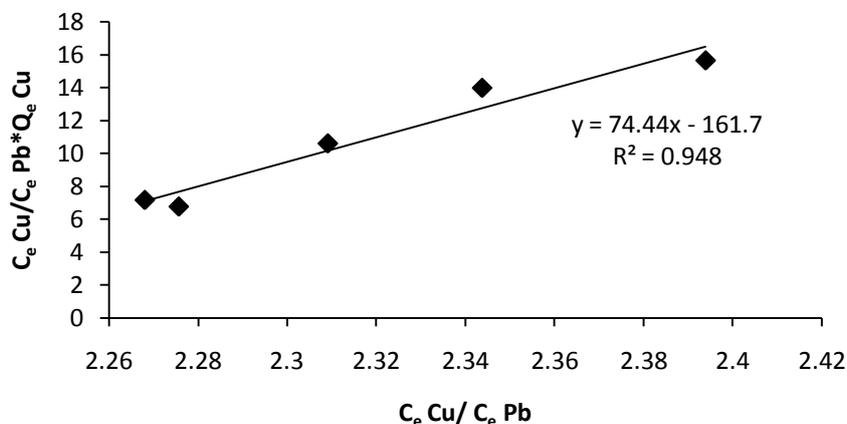
Figure 10: Cu-Pb binary sorption on baobab fruit shells
