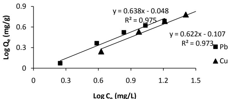
Figure 8: Freundlich isotherms for the adsorption of Pb<sup>2+</sup> and Cu<sup>2+</sup> on shells of baobab
