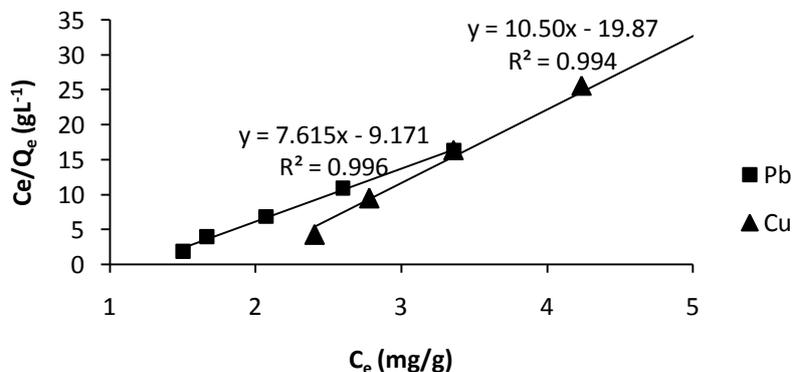
Figure 7: Langmuir isotherm for the adsorption of Pb<sup>2+</sup> and Cu<sup>2+</sup> on shells of baobab
