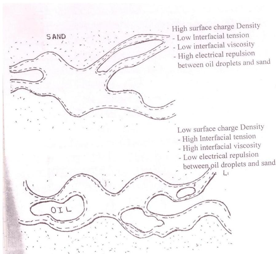
**Figure-6** The effect of surface charge density of oil\brine interface on the oil displacement process
