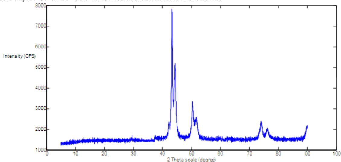
Figure 1 XRD pattern of CuNi nanoparticles
