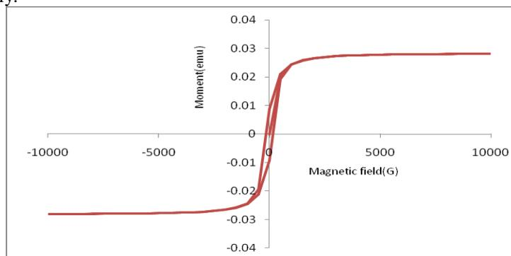
Figure 4 M-H Curves of CuNi nanoparticles
