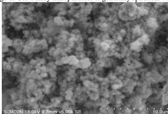
Figure 2 SEM image of CuNi nanoparticle
