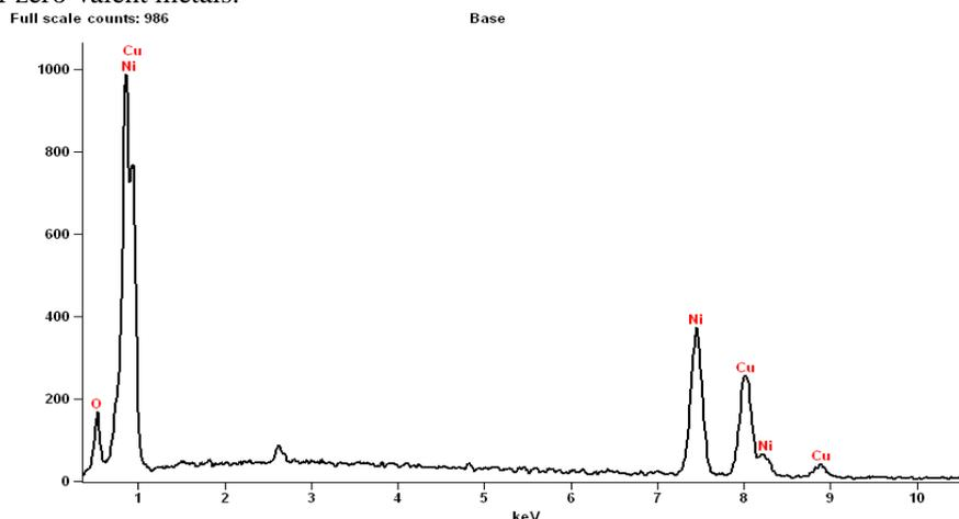
Figure 3 EDS image of CuNi Nanoparticles
