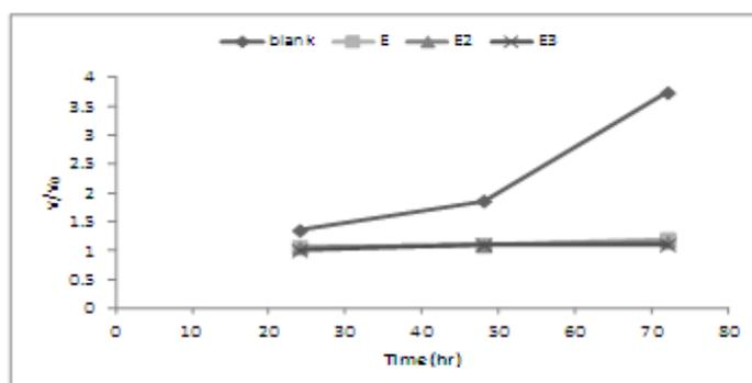
**Figure (8):** Variation of V/Vo with oxidation time of lube oil with additives of sulfur ratio = 1.5% with different basicity (E=neutral, E<sub>2</sub>=basic and E<sub>3</sub>=overbasic).
