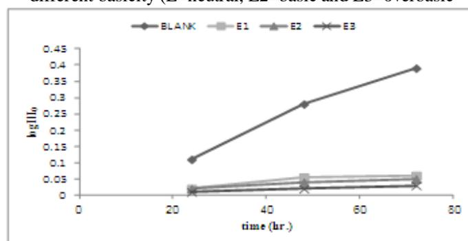
**Figure (10):** Variation of Log I/Io with oxidation time of lube oil with additives of sulfur ratio = 1.5% with different basicity (E=neutral, E<sub>2</sub>=basic and E<sub>3</sub>=overbasic).
