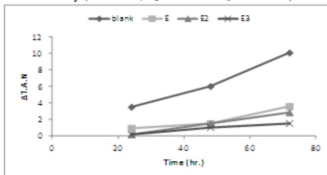
**Figure (9):** Variation of T.A.N. with oxidation time of lube oil with additives of sulfur ratio = 1.5% with different basicity (E=neutral, E<sub>2</sub>=basic and E<sub>3</sub>=overbasic)
