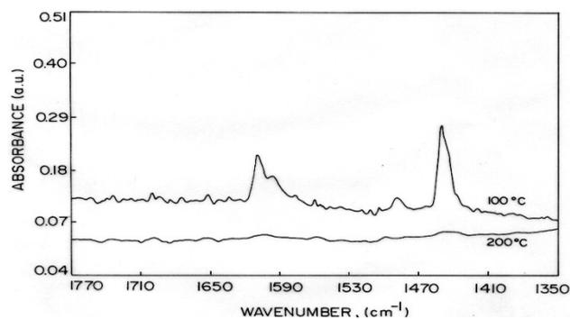
Fig. 2: IR of chemisorbed pyridine of Fe/Mi/SiO<sub>2</sub>.
