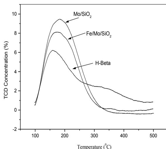
Fig. 4: TPD of ammonia of H-beta, Fe/Mo/SiO<sub>2</sub> and Mo/SiO<sub>2</sub> catalysts.
