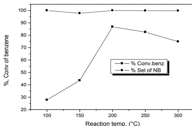
**Fig. 7:** Effect of temperature over Fe/Mo/SiO<sub>2</sub> catalyst.
