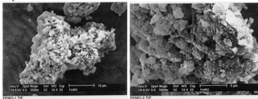
Fig. 3: Scanning electron micrograph of Fe/Mo/SiO<sub>2</sub>.
