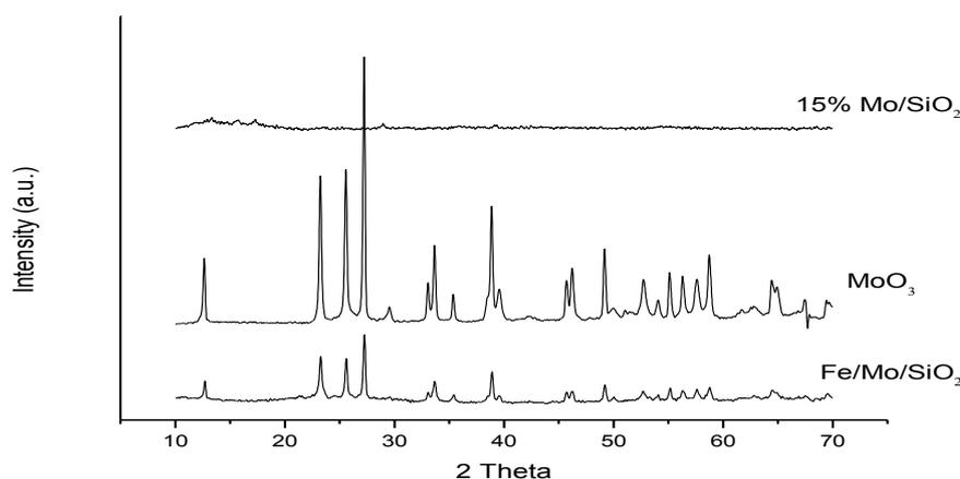
Fig. 1: XRD of Fe/Mo/SiO<sub>2</sub> and MoO<sub>3</sub>
