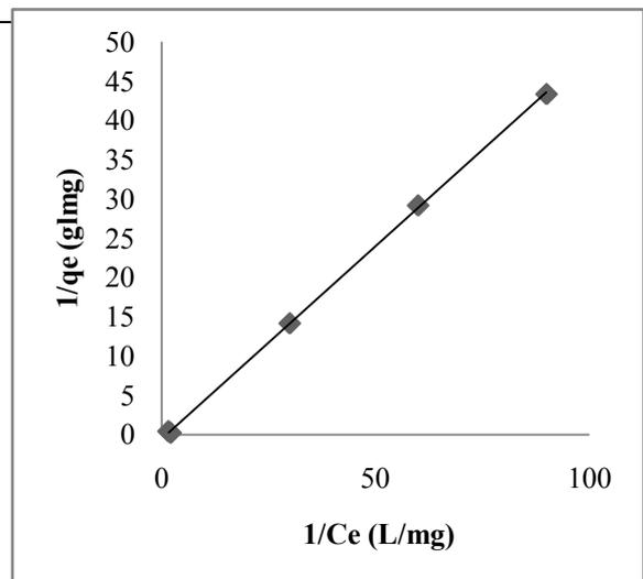
**Fig.4:** Langmuir isotherm for the adsorption of Pb<sup>2+</sup> by adsorbent, pH7 at 30 ±2<sup>o</sup>C.
