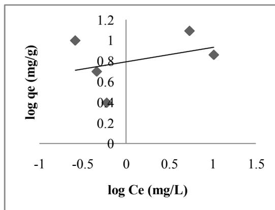
**Fig.5:** Freundlich isotherm for the adsorption of Pb<sup>2+</sup> by native pulverized locust beans hull, pH7 at 30±2<sup>o</sup>C.
