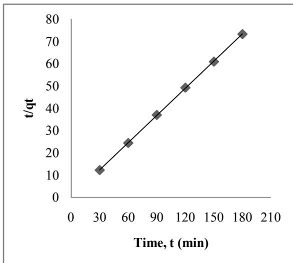
**Fig.3:** Pseudo-second-order for the adsorption of Pb<sup>2+</sup> by pulverized locust beans hull, pH 7 at 30±2<sup>o</sup>C
