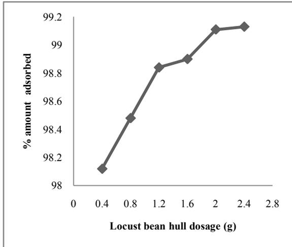
**Fig.1:** Influence of adsorbent dosage on Pb<sup>2+</sup> sorption, pH 7 at 30±2<sup>o</sup>C.
