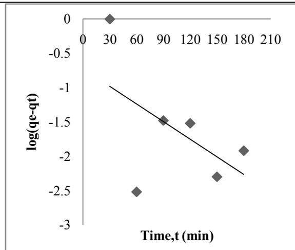
**Fig.2:** Pseudo-first-order for the adsorption of Pb<sup>2+</sup> by native pulverized locust beans hull, pH7 at 30±2<sup>o</sup>C.
