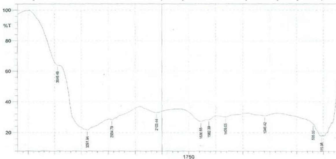
**Fig 1: FTIR of Unmodified Soybean Adhesive**
