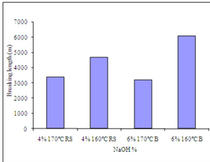
Fig. (2): Effect of pulping temperature on breaking length of rice straw and bagasse pulp.
