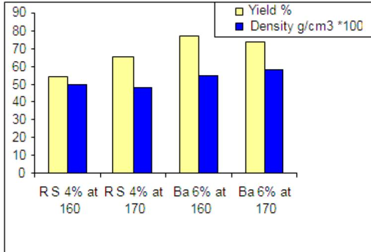
Fig. (1): Effect of pulping temperature on the yield and density
