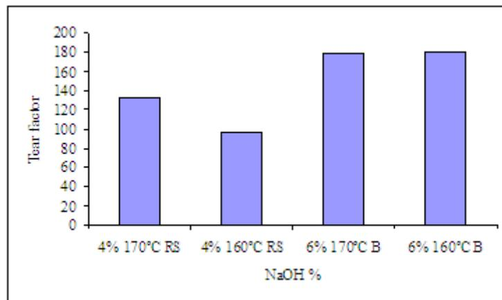
Fig. (3): Effect of pulping temperature on tear factor of rice straw and bagasse pulp.
