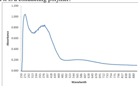
**Fig 2** UV-Visible spectrum of Polyaniline
