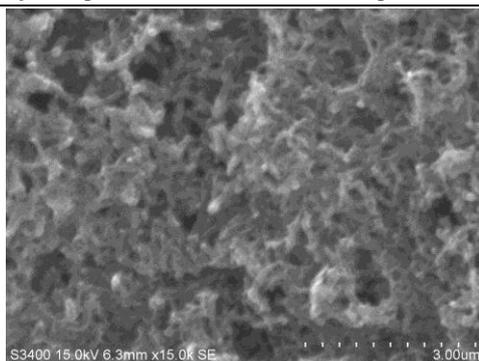
**Fig. 5** SEM image of Polyaniline
