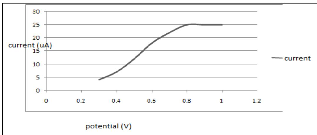
Fig 9 Current–potential curves for the PANI-2AP-GOD electrode in 0.1 M phosphate buffer, pH 7.0.
