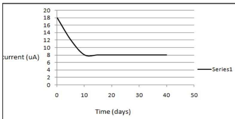
Fig 10 Stability of the PANI-2AP-GOD electrode on storage in 0.1 M phosphate buffer, pH 7.0
