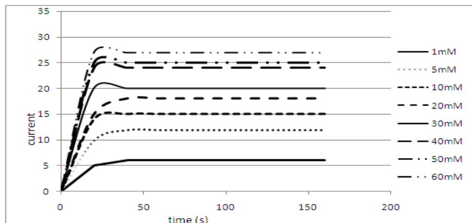
Fig 5. Current–time curve during the PANI-2AP-GOD electrode at 0.7 V and pH 7.0 in 0.1 M phosphate buffer for different glucose solution of 1–50 mM.
