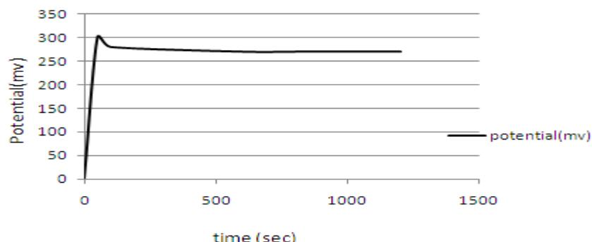
Fig.1 Current–time curve during the synthesis of PANI-2AP film in aqueous solution At current density 1 mA/cm<sup>2</sup> and pH 3.0
