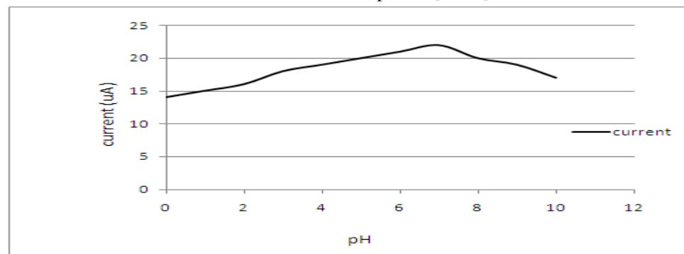
Fig 8 . Effect of pH on the GOD electrode response of PANI-2AP. Steady currents measure at 0.7 V in 5 mM glucose solution in 0.1 M phosphate buffer
