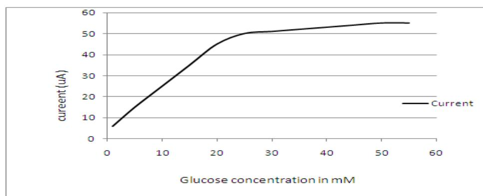
Fig 6 The relationship between response current and glucose concentration for the PANI-2AP-GOD electrode in 0.1 M phosphate buffer, pH 7.0
