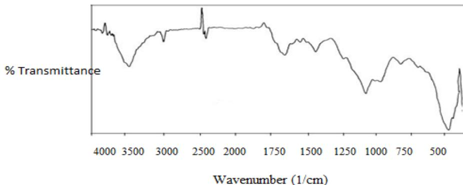
Fig 3 . FT-IR spectra of PANI-2AP film in aqueous solution at current density 1 mA/cm<sup>2</sup> and pH 3.0.
