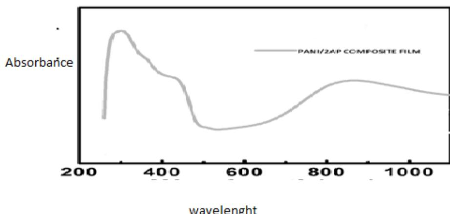
Fig 2 UV–Vis spectra of PANI-2AP film in aqueous solution at current density 1 mA/cm<sup>2</sup> and pH 3.0.
