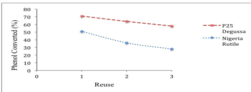
**Figure 9:** The reusability of Nigeria rutile compare with P25 Degussa in the Photocatalytic Degradation of Phenol
