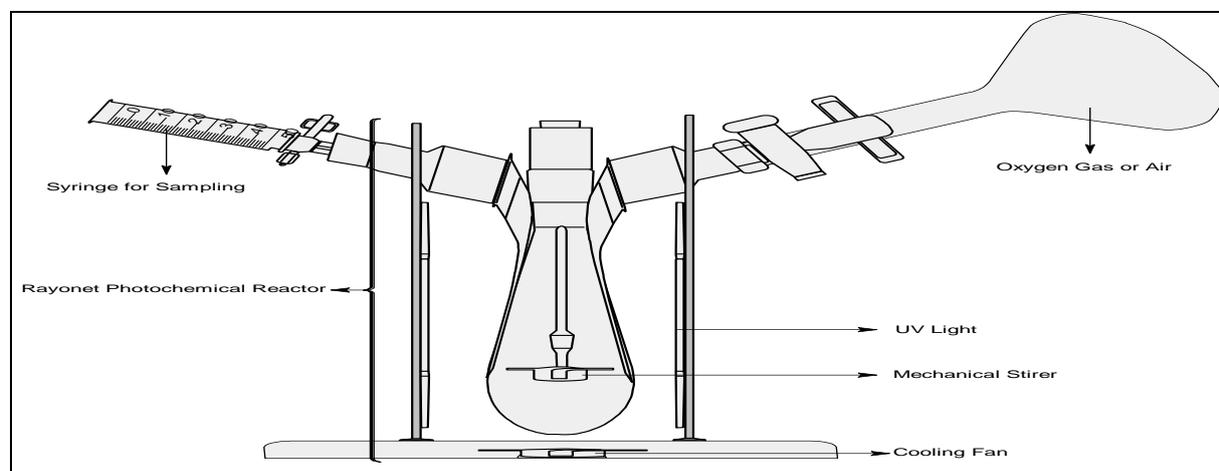
Figure.1. Diagram of the Photo catalytic Set-up
