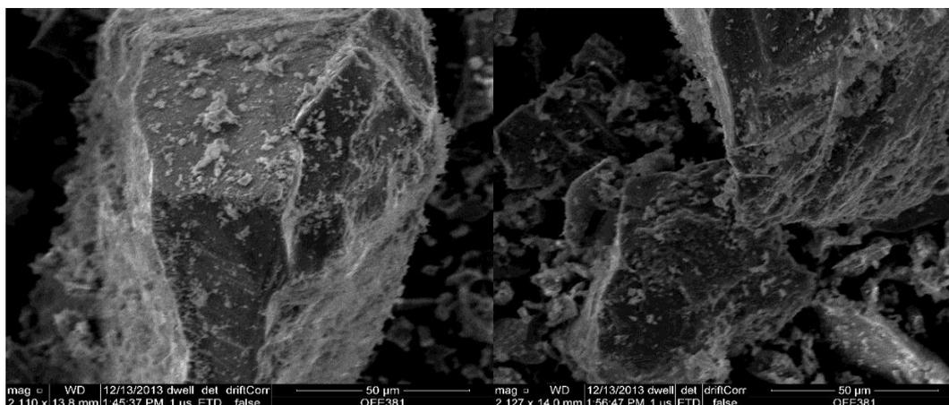
**Figure 5.** Scanning electron microscopic photograph of the rutile from the Middle Belt region of Nigeria.
