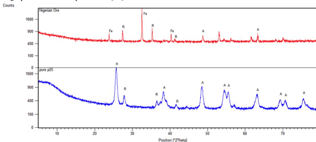
**Figure 4.** X-ray diffraction patterns of the Nigerian rutile and P25 Degussa
