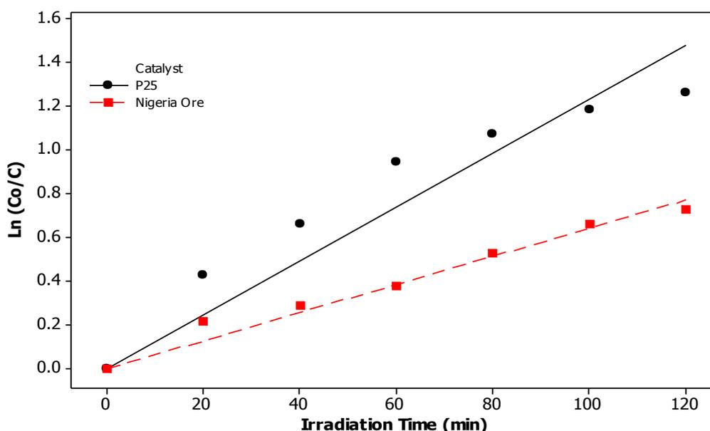
**Figure 7.** The Linear fit to the data represent Pseudo-first-order degradation kinetics of P25 and Nigeria rutile.
