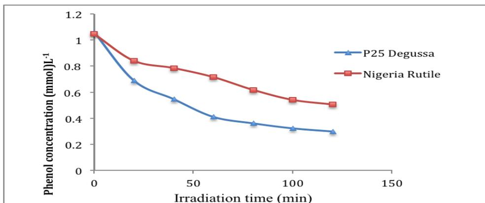
**Figure 8:** Phenol degradation in present of Nigeria rutile and P25 Degussa in UV light with Oxygen
