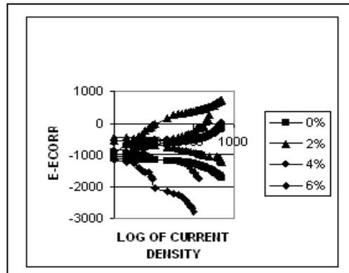
Fig 9: Potentiostat test in 3.5 % sodium chlorides solution
