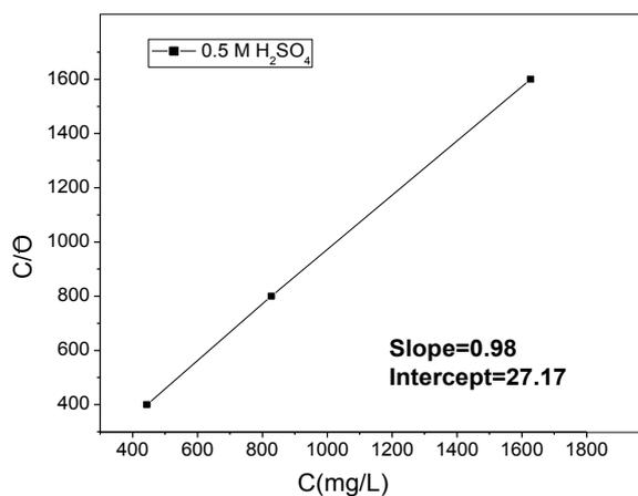
Fig 4. Langmuir adsorption isotherm for water extract of SM on mild steel in 0.5 M H<sub>2</sub>SO<sub>4</sub>.
