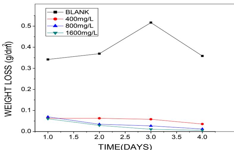
Fig 1 : Weight loss against time for mild steel in 0.5 M H<sub>2</sub>SO<sub>4</sub> in the absence and presence of 400 mg/L, 800 mg/L and 1600 mg/L of water extract of SM leaves.
