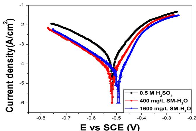
Fig 3 Potentiodynamic polarization curves for mild steel in 0.5 M H<sub>2</sub>SO<sub>4</sub> in the absence and presence of 400mg/L and 1600mg/L SM- water extract.
