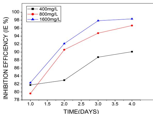
Fig 2: Inhibition efficiency against time for mild steel in 0.5 M H<sub>2</sub>SO<sub>4</sub> containing 400 mg/L, 800 mg/L and 1600 mg/L of water extract of SM leaves.
