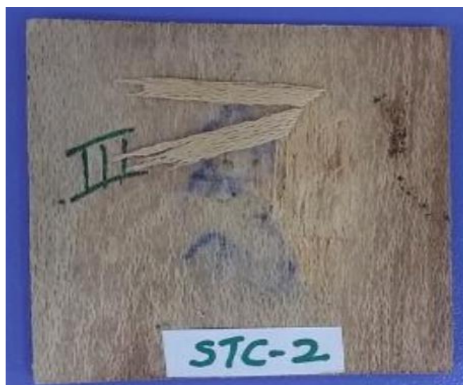
Plate 2 Wet bond strength of adhesive IV coated plywood as per IS 848-2006 for BWP grade
