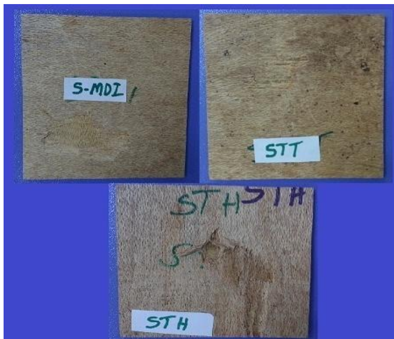
Plate 1 Dry Bond strength of SMDI, STT and STH without cyclic test
