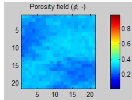
**Fig.2** Porosity distribution of reservoir model
