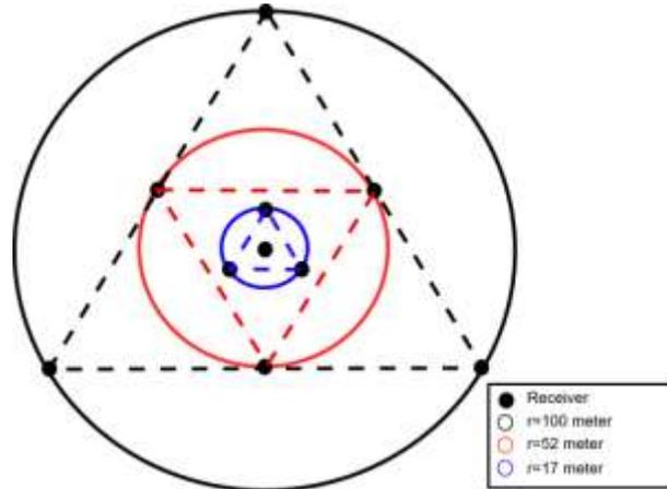
Fig. 2: Survey plan of SPAC measurement
