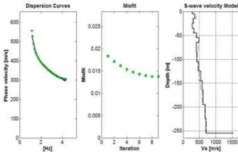
Fig. 5: Dispersion curve, misfit and vertical S-wave velocity structure for K2 measurement point.
