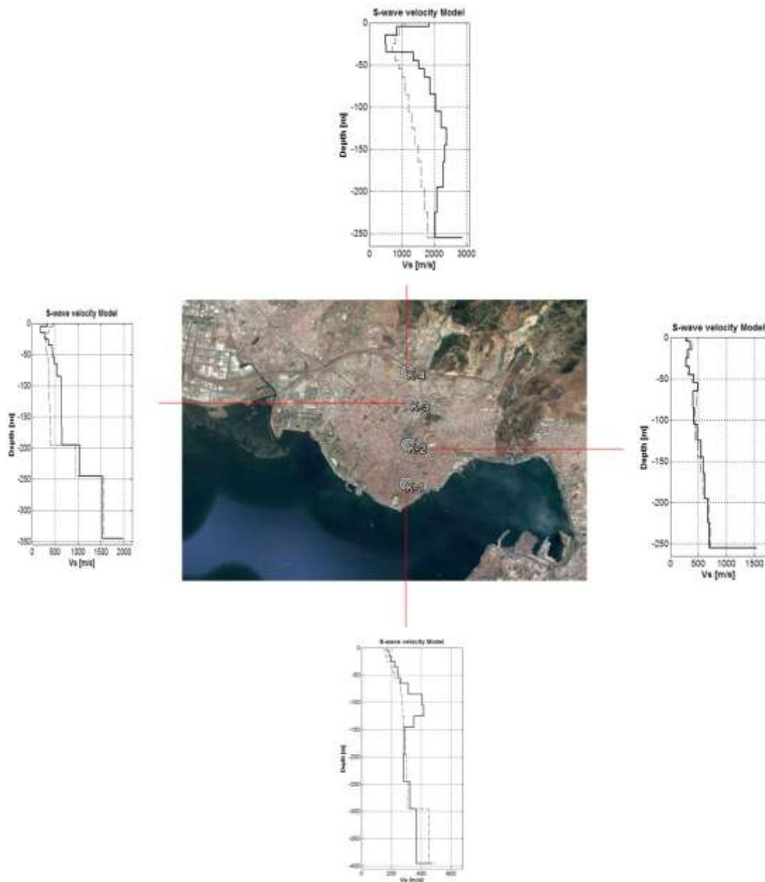
**Fig. 8:** Summarizing of S-wave vertical velocity models for all measurement points
