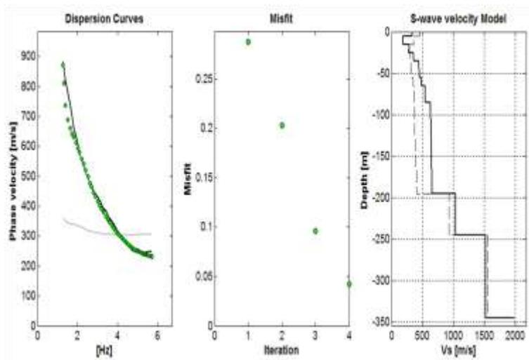
Fig. 6: Dispersion curve, misfit and vertical S-wave velocity structure for K3 measurement point.
