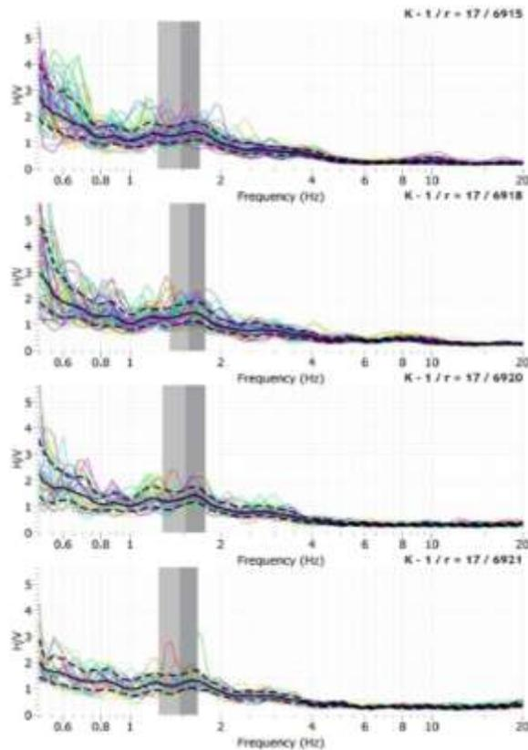
Fig. 8: Horizontal to vertical spectral ratio (HVSr) result for Karsiyaka at K1 SPAC point using 17 m criteria.
