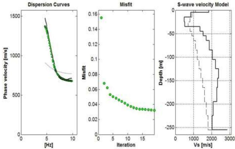
Fig. 7: Dispersion curve, misfit and vertical S-wave velocity structure for K4 measurement point.
